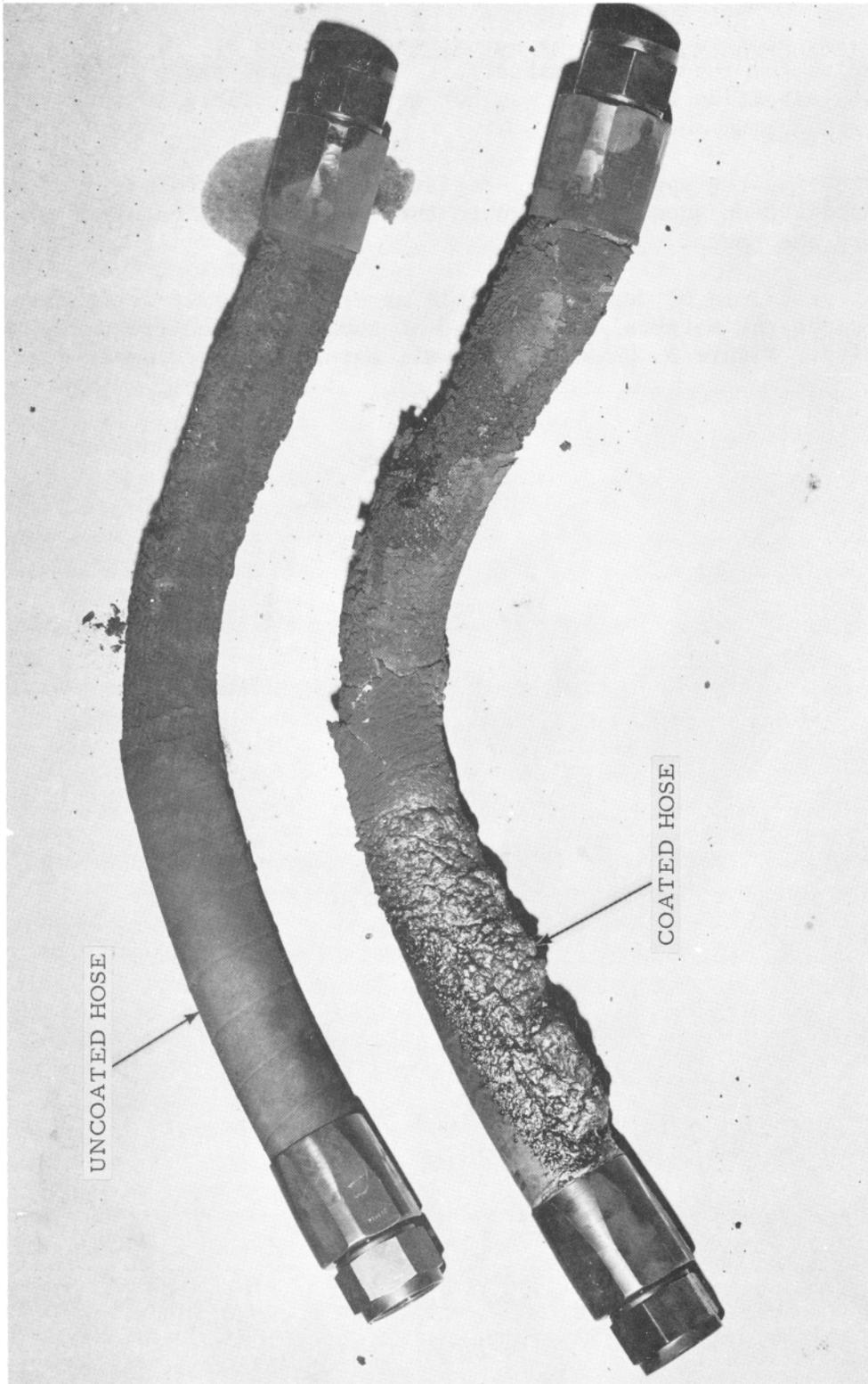
FIGURE 8. DAMAGE TO HOSE SPECIMENS
