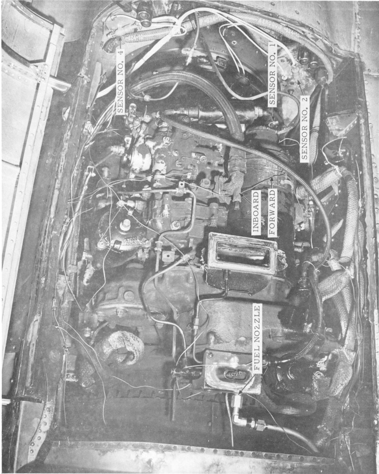
FIGURE 4. FUEL-TO-FIRE NOZZLE AT THE 6 O'CLOCK POSITION,
