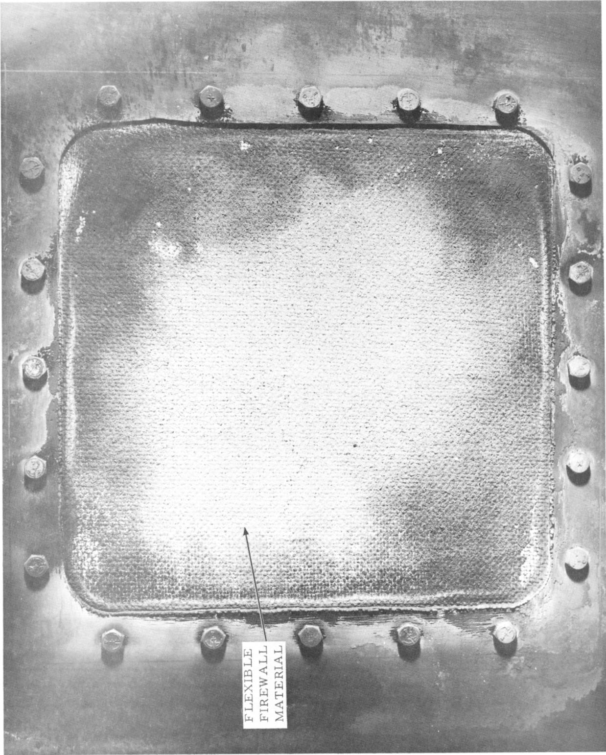
FIGURE 9. FIREWALL MATERIAL AFTER 2,000°F TESTS
