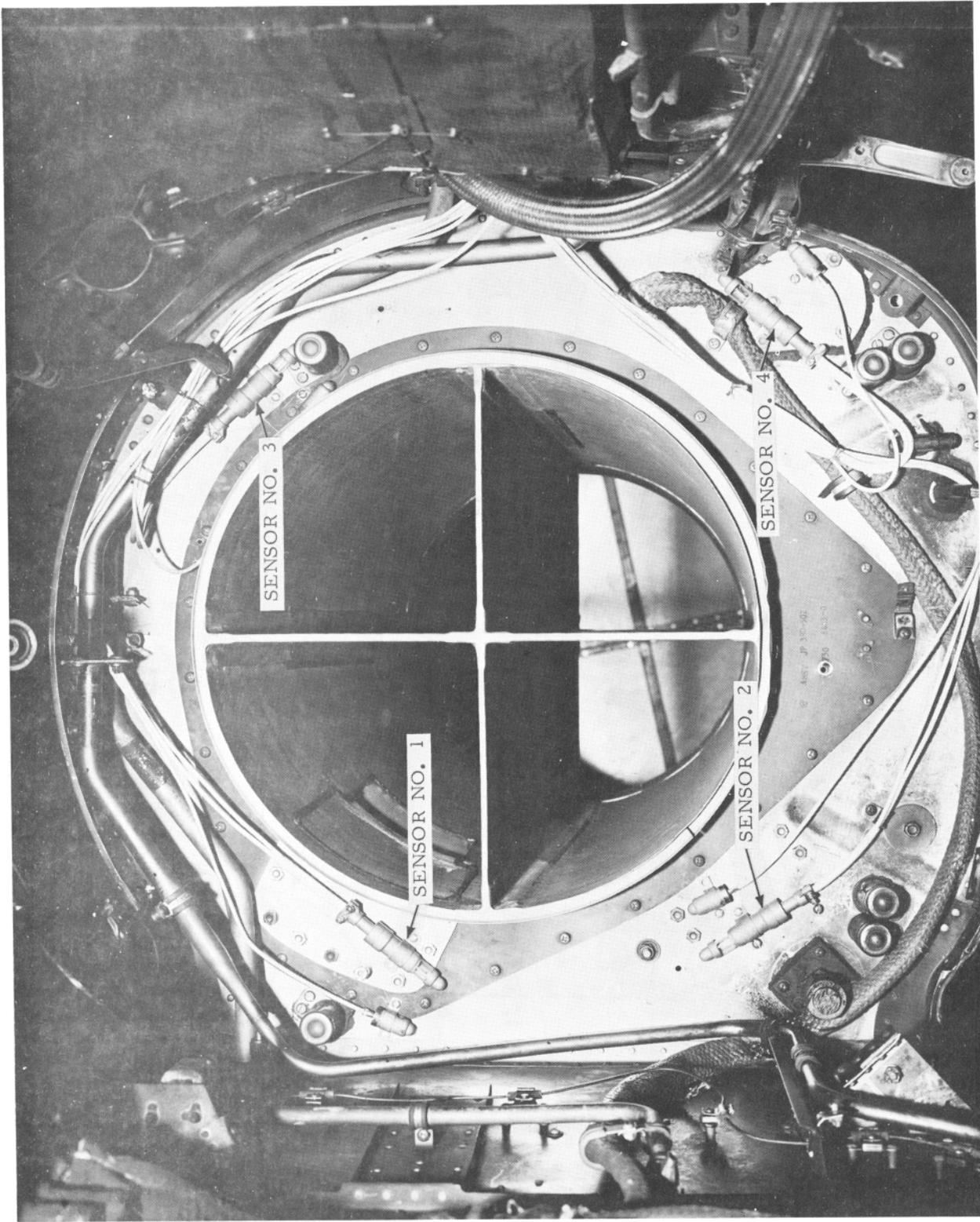
FIGURE 2. EDISON UV SENSOR INSTALLATION ON FORWARD BULKHEAD OF NACELLE
