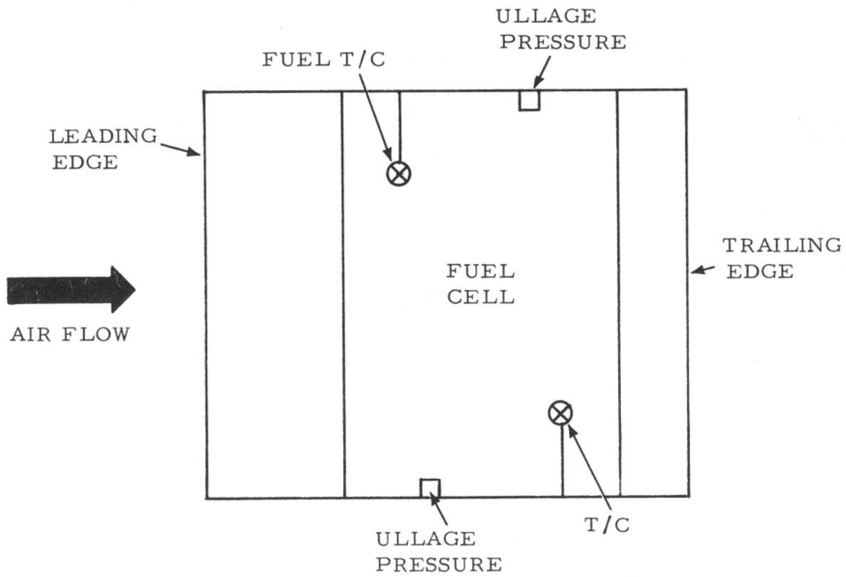
FIGURE 15. INSTRUMENTATION IN THE VERTICAL TEST ARTICLE
