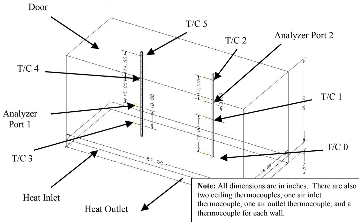
FIGURE 2. THERMOCOUPLE AND ANALYZER PORT LOCATIONS
