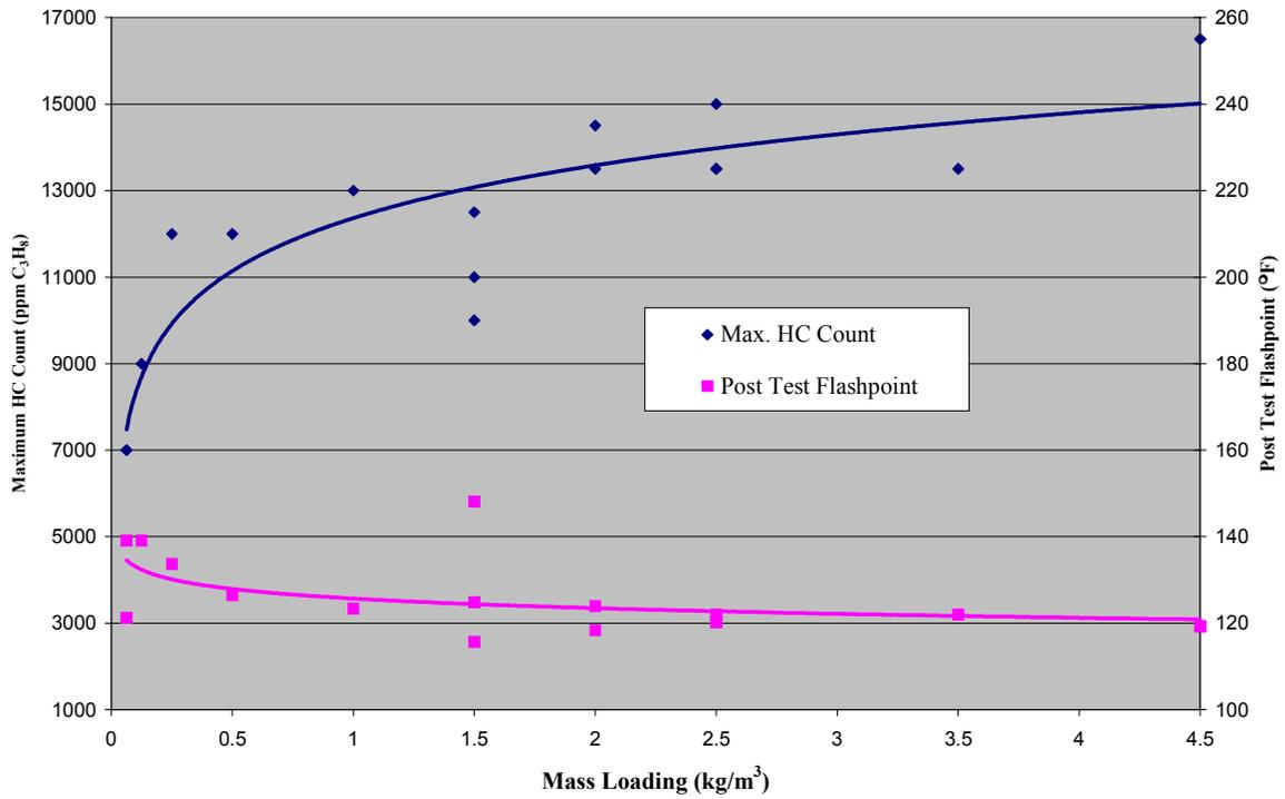
FIGURE 3. MAXIMUM HYDROCARBON COUNT (ppm C<sub>3</sub>H<sub>8</sub>) AND POSTTEST FLASHPOINT (°F) AS A FUNCTION OF MASS LOADING
