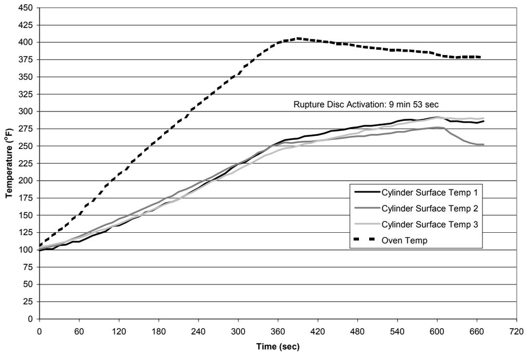
FIGURE 2. FURNACE TEST RESULTS USING A 76.5-CUBIC-FOOT CYLINDER
