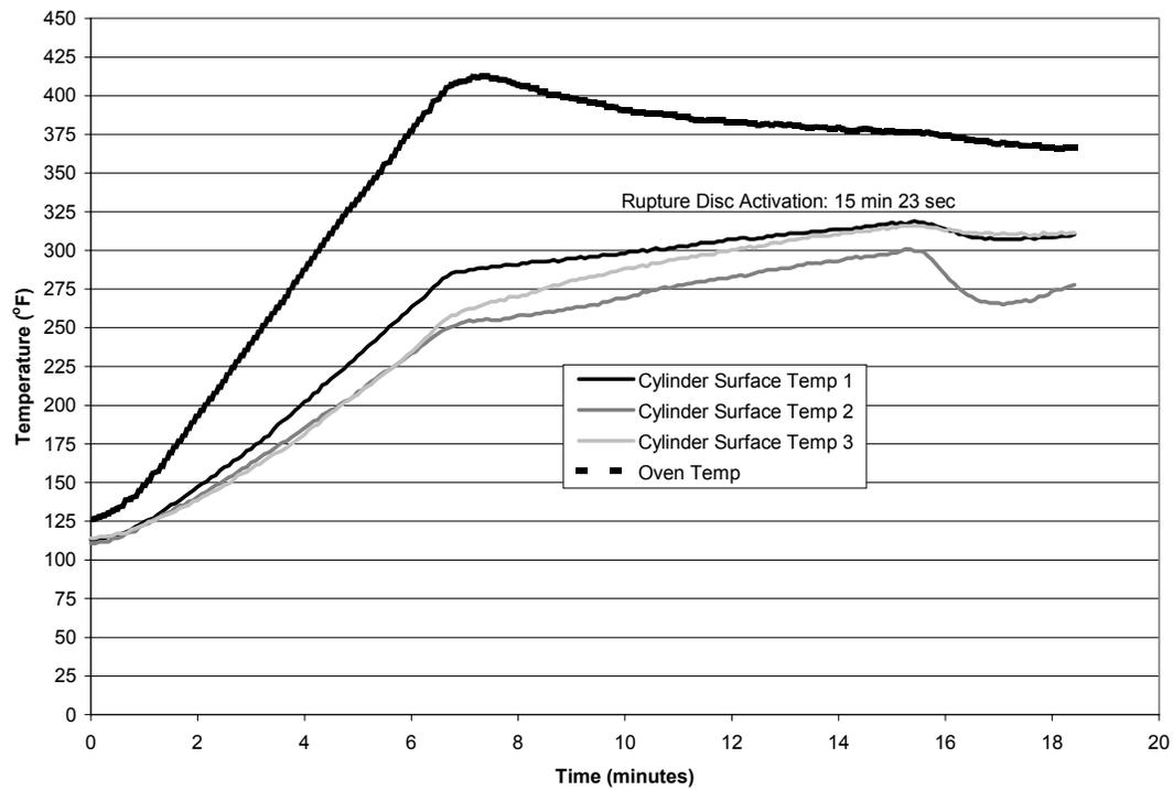
FIGURE 3. FURNACE TEST RESULTS USING A 115-CUBIC-FOOT CYLINDER
