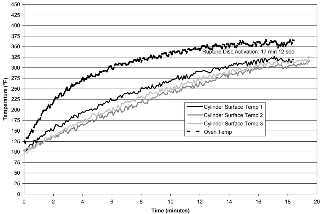
FIGURE 4. FURNACE TEST RESULTS USING AN 11-CUBIC-FOOT CYLINDER
