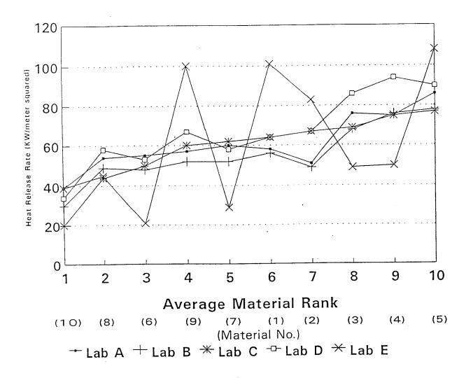
FIGURE 2. AVERAGE PEAK HEAT RELEASE RATE FOR TEN MATERIALS
