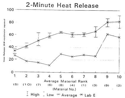
FIGURE 1. AVERAGE TOTAL HEAT RELEASE AT TWO MINUTES FOR TEN MATERIALS
