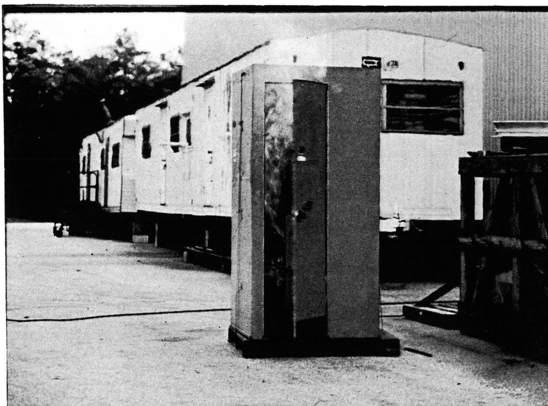
FIGURE 2. BUTANE IGNITED INSIDE LAVATORY (1 of 3 Sheets)
