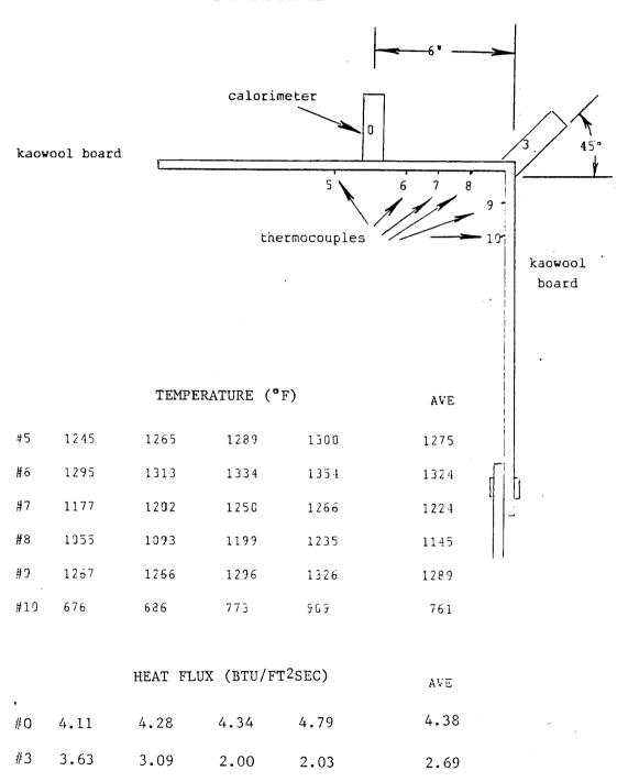
FIGURE 4. CORNER FLAME INTENSITY MEASURING APPARATUS (PROPANE)
