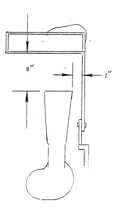
FIGURE 3. RELATIVE POSITIONS OF BURNERS
