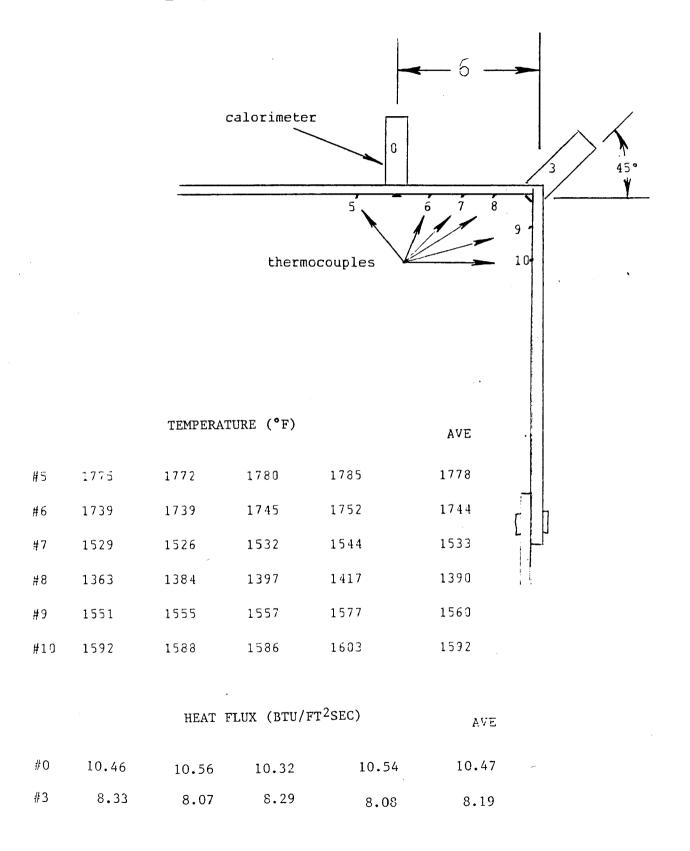
FIGURE 5. CORNER FLAME INTENSITY MEASURING APPARATUS (KEROSENE)
