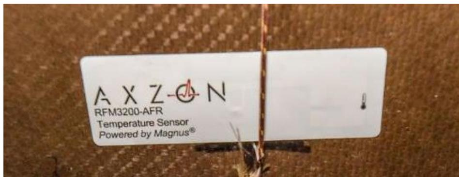
*Figure 13 Axzon RFM3200-AFR Temperature Sensing RFID Tag*
