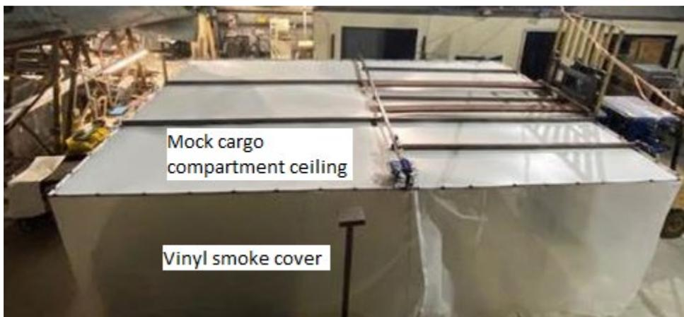
*Figure 11 Design of Mock Cargo Compartment Ceiling with Vinyl Smoke Cover*
