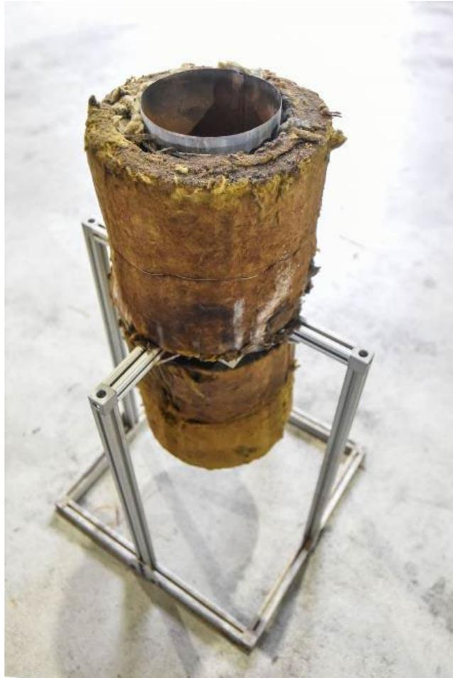
*Figure 8 Insulated Aluminum Pipe Containing Wood Pellets for Smoldering*
