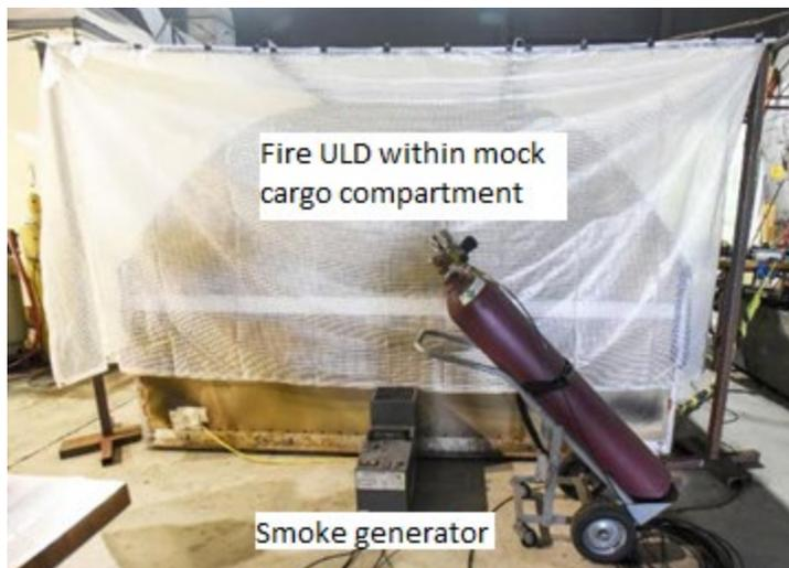
*Figure 7 Aviator 440 Smoke Generator Piped into Fire ULD*
