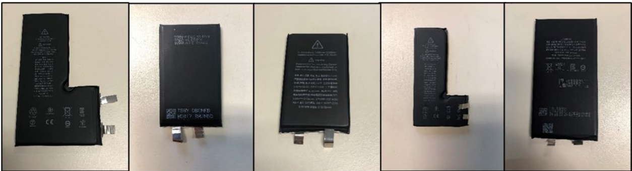
Figure 1. Battery Cells from left to right; 3.79V, 3.80V Cell #1, 3.80V Cell #2, 3.83 L-Shaped, 3.83 Square
