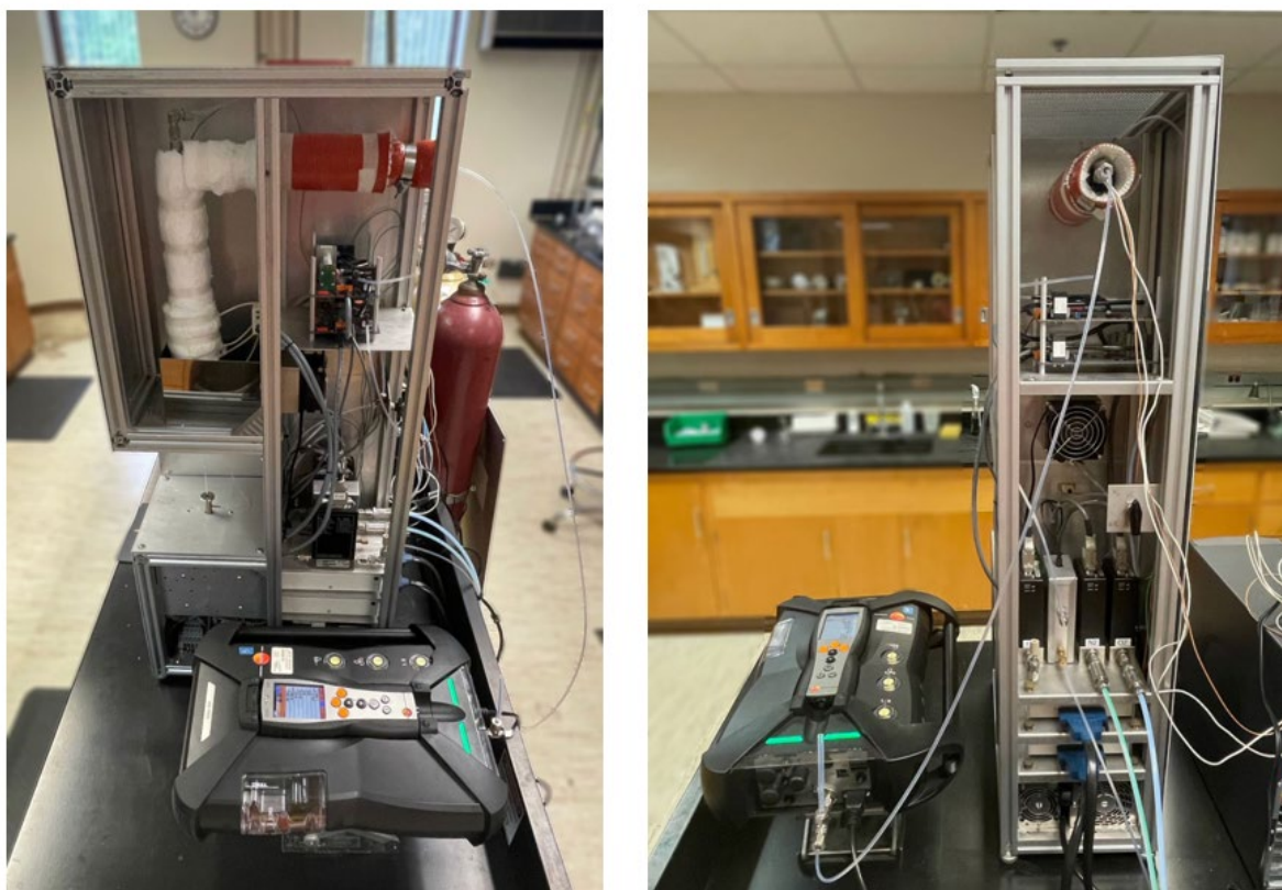
Figure 6. Testo multigas analyzer connected to MCC exhaust
