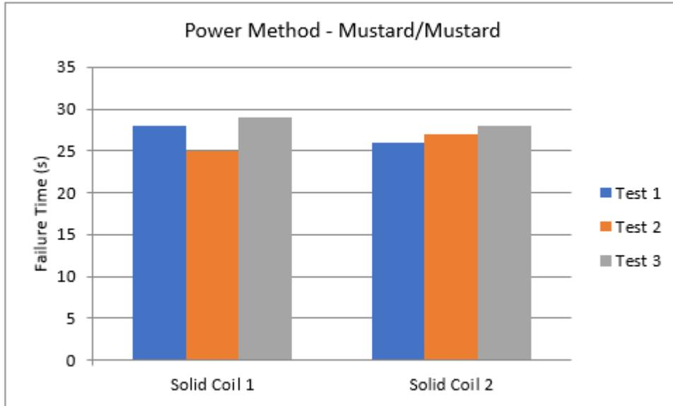
Figure 21. Comparing two solid coils using Mustard/Mustard materia
