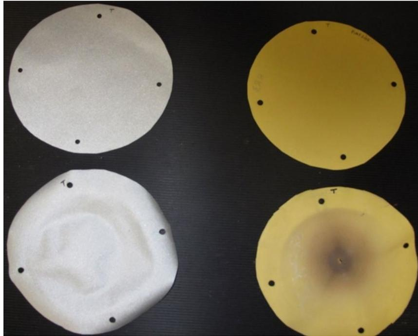
Figure 6. Yellow/Gray (left) and Mustard/Mustard materials (right) before and after a test
