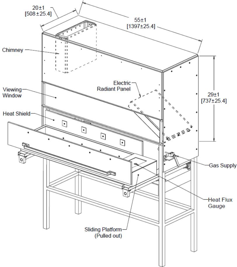
Figure 1. Diagram of the radiant panel insulation test apparatus
