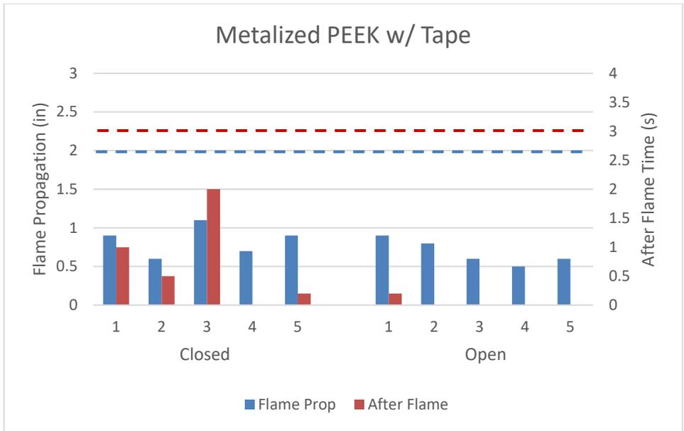
Figure 4. Metalized PEEK with metalized PEEK tape test results
