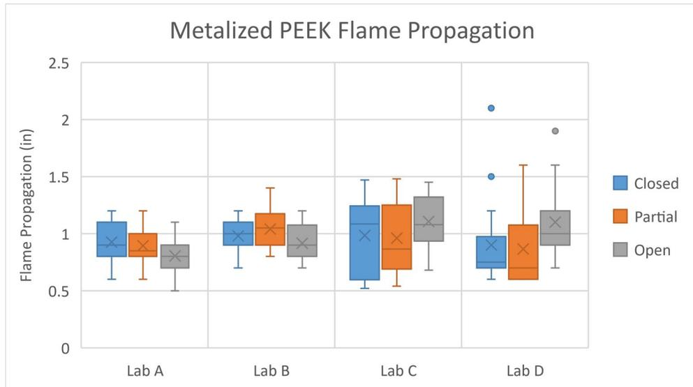
Figure 14. Box and whisker plot of flame propagation
