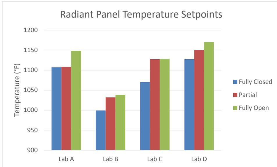
Figure 10. Radiant Panel temperature set points to reach calibration at each gap setting
