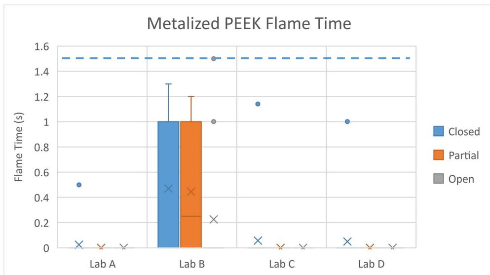
Figure 15. Box and whisker plot of after flame time
