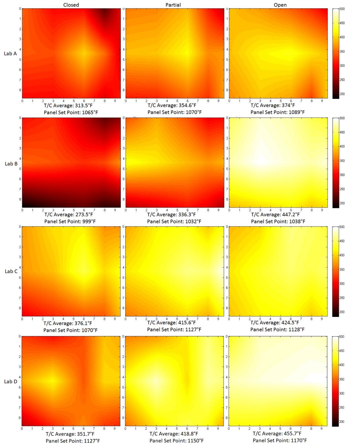
Figure 11. Heat maps from thermocouple array on top surface of drawer
