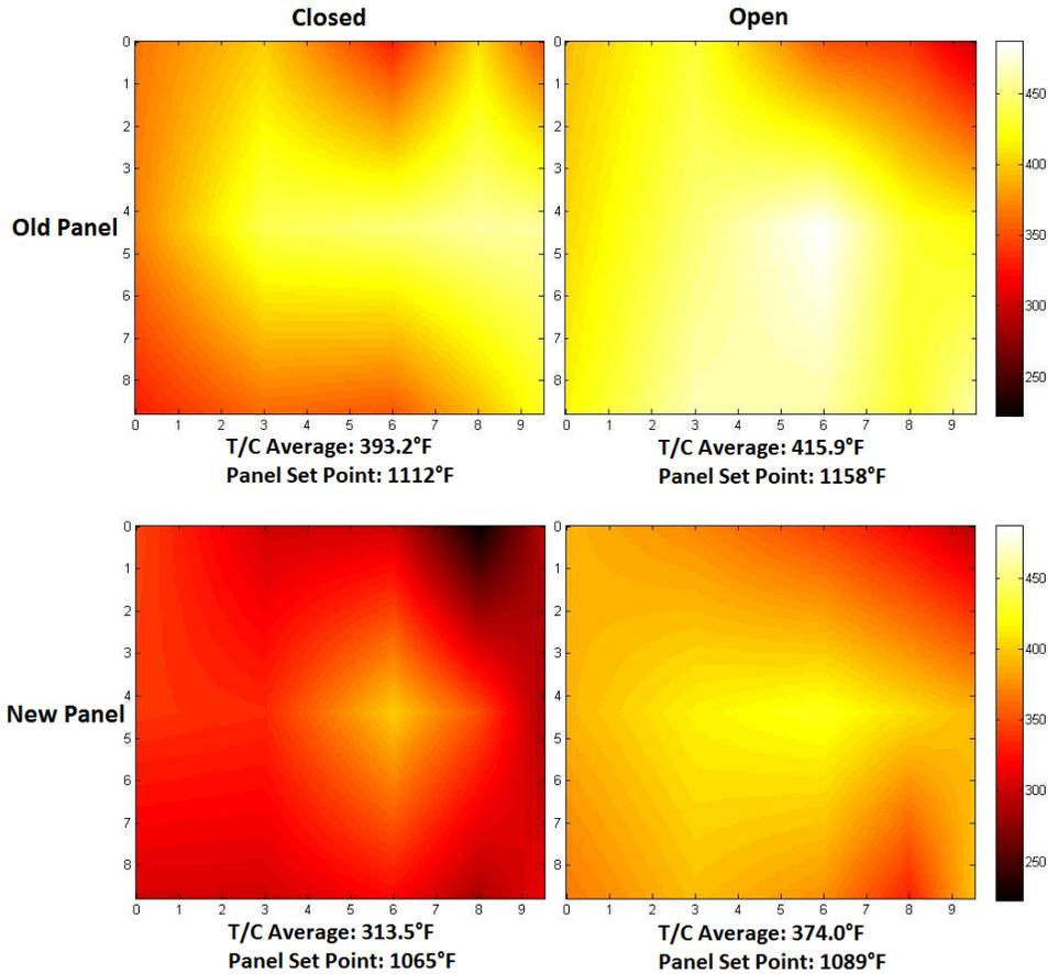
Figure 12. FAA's old panel compared to new panel
