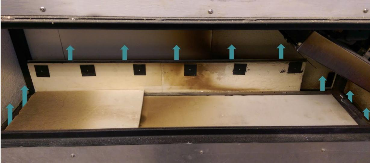
Figure 2. Blue arrows indicate where room temperature air enters the chamber
