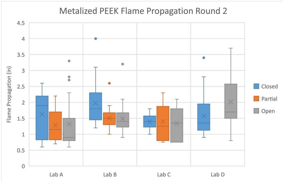
Figure 23. Box and whisker plot of round two flame propagation
