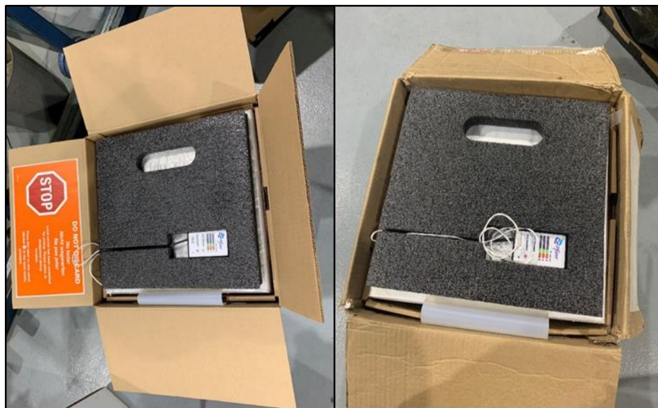
Figure 9. Medium Type B container damages
