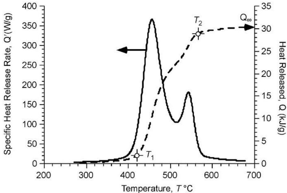
Figure 5. Specific Heat Release Rate and its Time Integral versus Temperature in the MCC Showing location of  $T_1$ ,  $T_2$ , and  $Q_\infty$  for Calculation of  $FGC$ .
