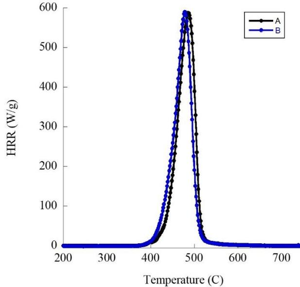
Figure A2. Specific Heat Release Rate Curves versus Temperature in MCC for Case Study #5
