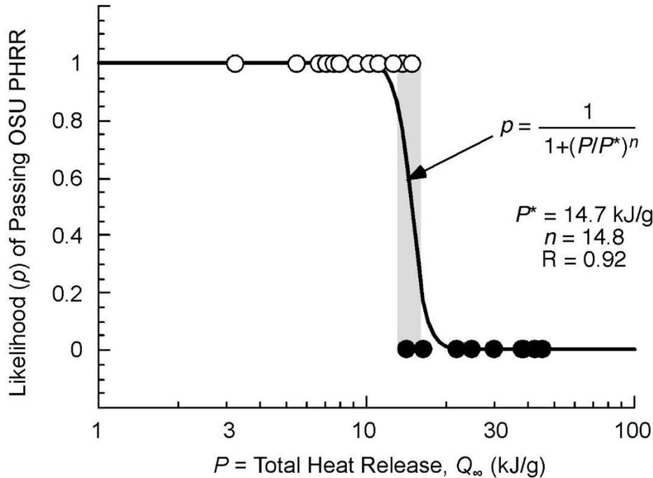
Figure 1. Likelihood of Passing  $PHRR$  versus  $Q_{\infty}$  of the 19 Polymers in Figure 2.
