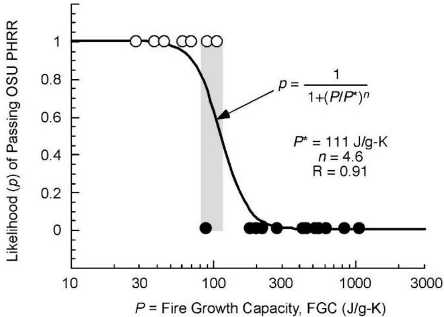
Figure 3. Likelihood of passing the *PHRR* versus *FGC* of the 19 polymers in Figure 2
