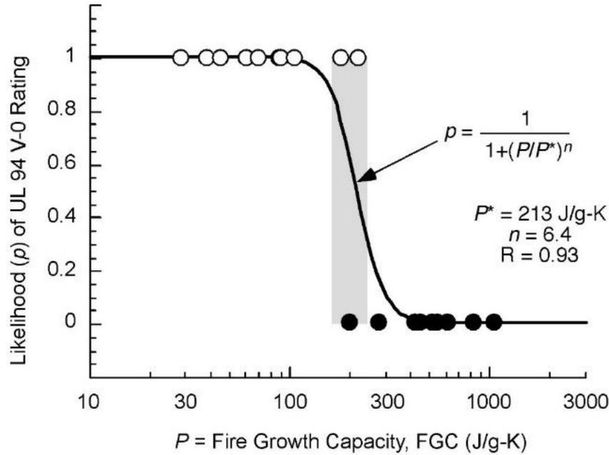
Figure 4. Likelihood of a UL 94 V-0 rating versus *FGC* for the 19 polymers in Figure 2
