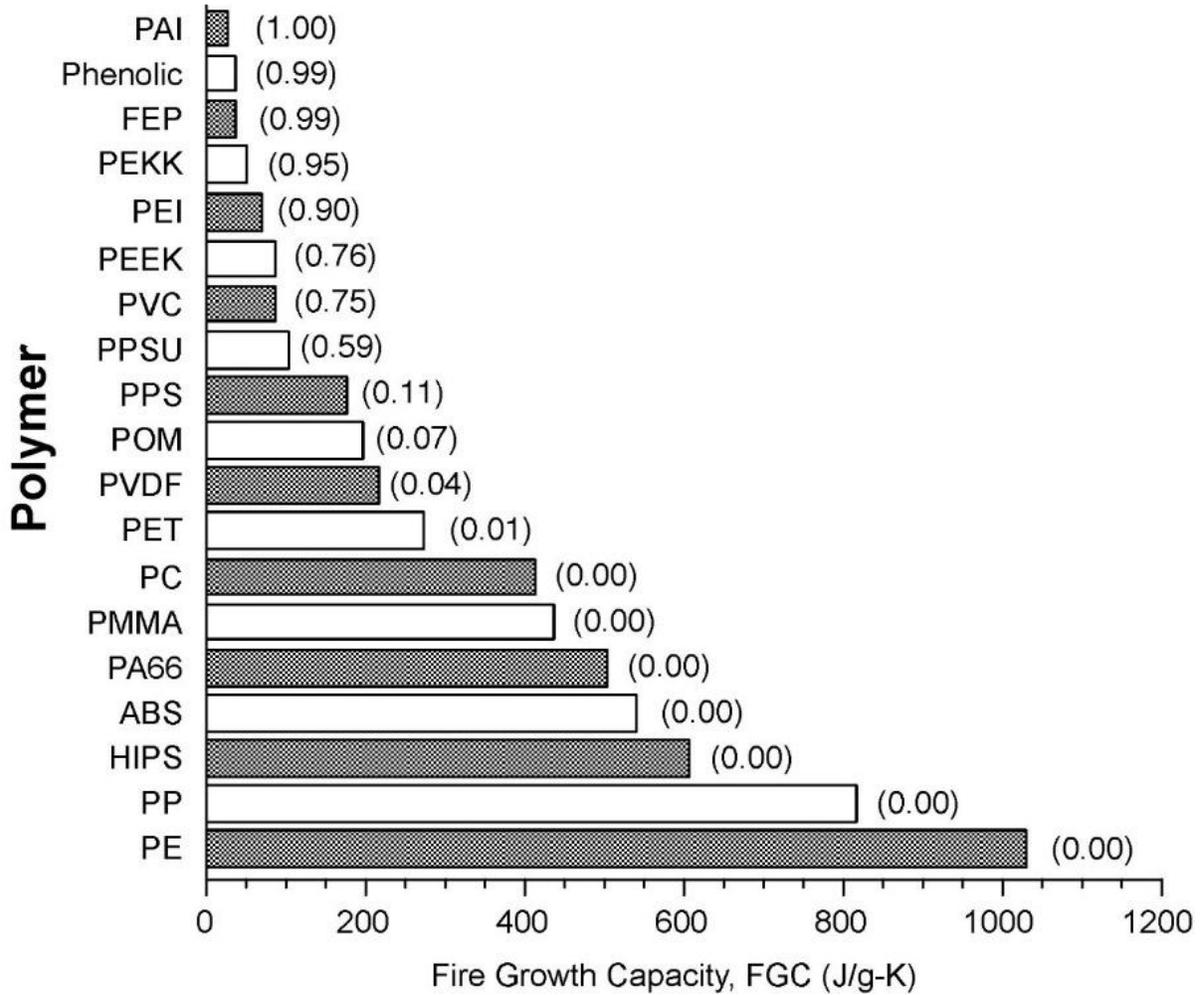
Figure 2. Fire Growth Capacities (FGC) of 19 commercial polymers
