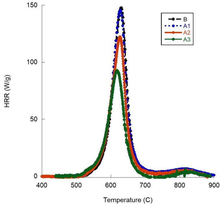
Figure A5. Specific Heat Release Rate Curves versus Temperature in MCC for Case Study #9
