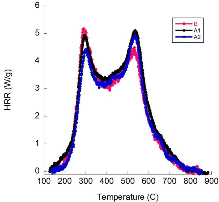
Figure A7. Specific Heat Release Rate Curves versus Temperature in MCC for Case Study #11
