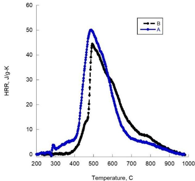
Figure A3. Specific Heat Release Rate Curves versus Temperature in MCC for Case Study #7
