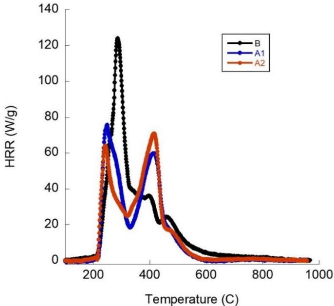
Figure A1. Specific Heat Release Rate Curves versus Temperature in MCC for Case Study #3
