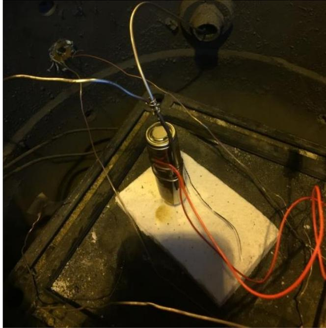
**Figure 5. Overheat setup – 18650 cell**
