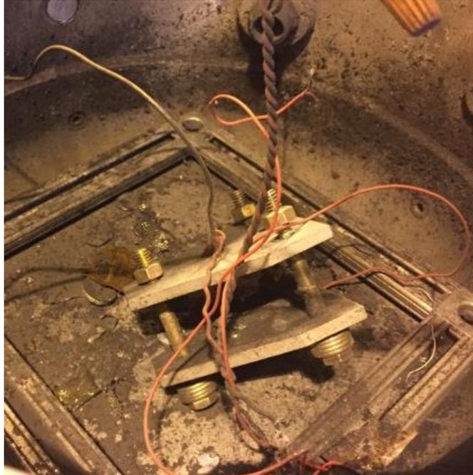
**Figure 10. Thermal runaway by overheating with battery holder assembly – CR123a cell**
