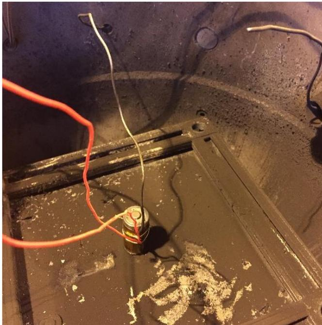
**Figure 3. Overheat without battery holder assembly – CR123a cell**
