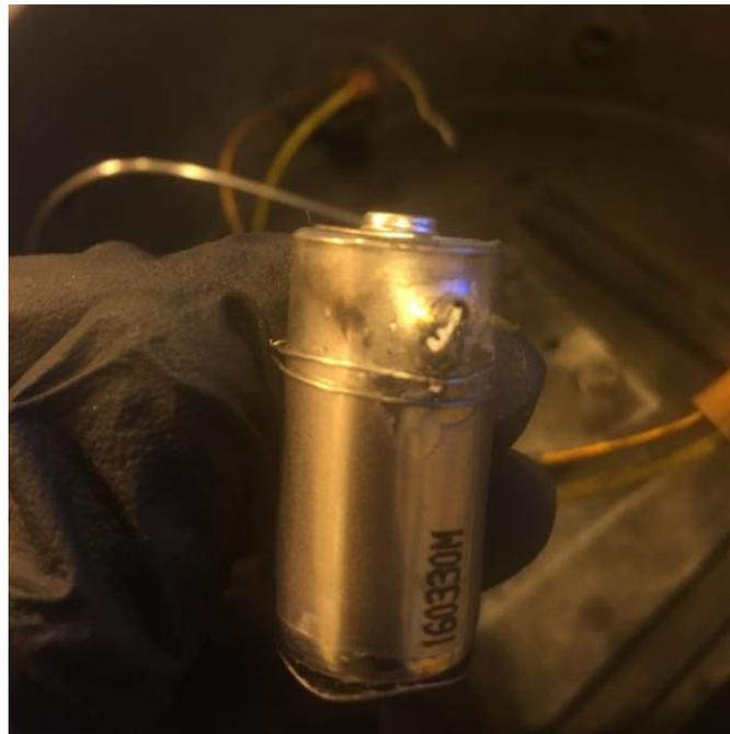
**Figure 12. Deformation of cell casing due to thermal runaway by overcharging – CR123a cell**
