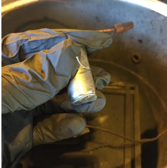
**Figure 13. Deformation of cell casing due to energetic failure by overcharging – CR123a cell**
