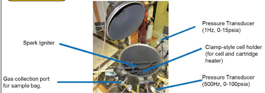
Figure 4. A 21.7 L test chamber for small-scale tests
