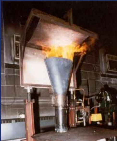
Cargo liner oil burner test
