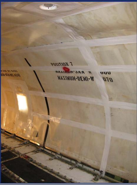
Class E Cargo Compartment Smoke Detection and Active ULD Testing
