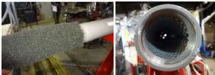
Muffler foam was removed
