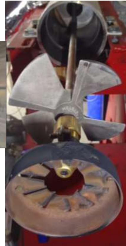
Added Carlin type turbulator on fuel nozzle fitting
