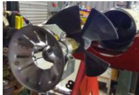
Added Carlin type turbulator on fuel nozzle fitting
