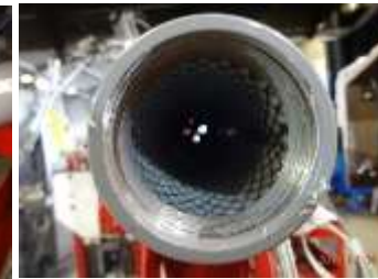
Muffler foam was removed
