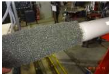
Muffler foam was removed
