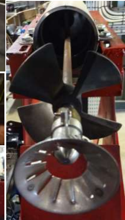
Added Carlin type turbulator on fuel nozzle fitting
