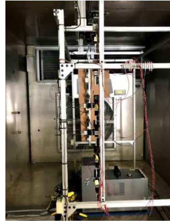
Thermocouples, anemometers, EMERSM and obscuration meters
