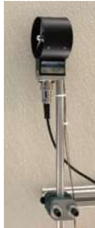
Vane anemometer cross-checked with hot film anemometer
