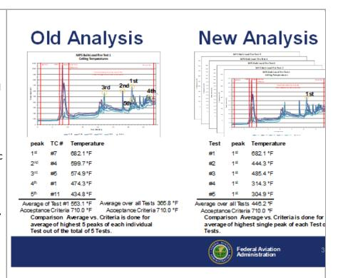
The acceptance criteria for the bulk-load fire scenario are that the average of the single highest peak temperature for each of the five tests shall not exceed 710°F (377°C), starting 2 minutes after the suppression system is initially activated until the end of the test. In addition, the average of the five tests areas under the time-temperature curve of the compartment thermocouples shall not exceed 9850°F-min(4974°C-min).
