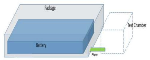
As an alternative to a complete package test, a sub-system may be tested instead. The sub-system shall consist of
