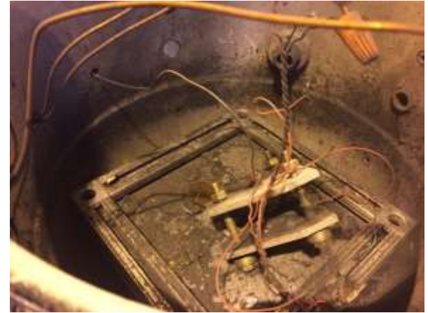
Fragmented battery after overheat method
