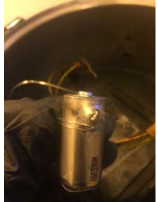
DC overcharge post thermal runaway
