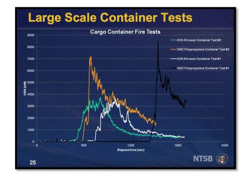
The peak heat release rate (HRR) <u>is more then twice as great</u> in a polypropylene ULD vs a standard ULD
