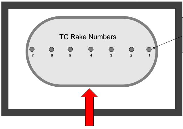
Thermocouples placed 1" above centerline with 1" spacing between each T/C
