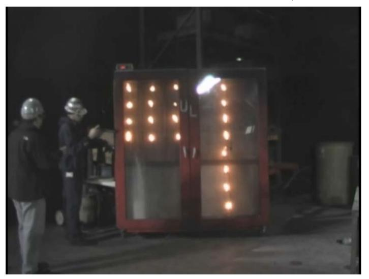
Passed FAA MPS AR-01/37 seat fire toxicity tests, February 2011
