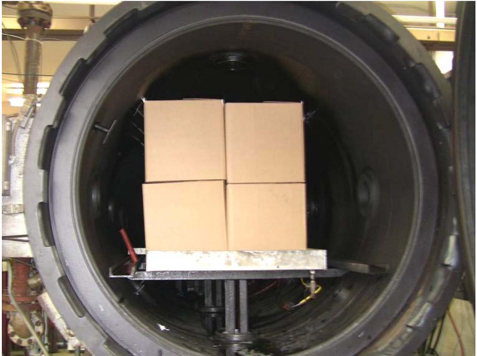
Cargo Fire Suppression by Depressurization Tests
