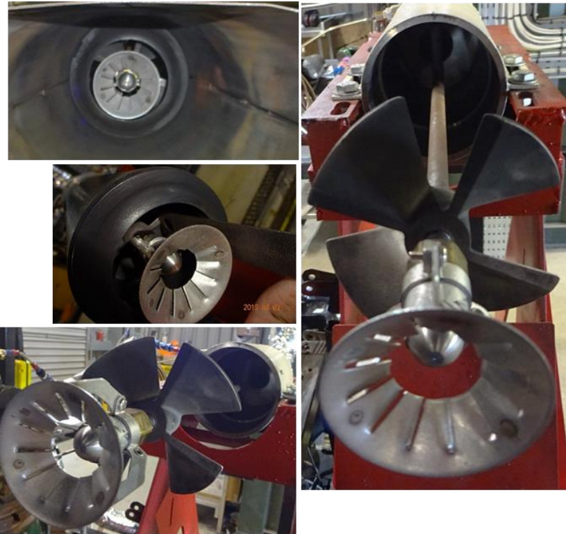
Added Carlin type turbulator on fuel nozzle fitting
