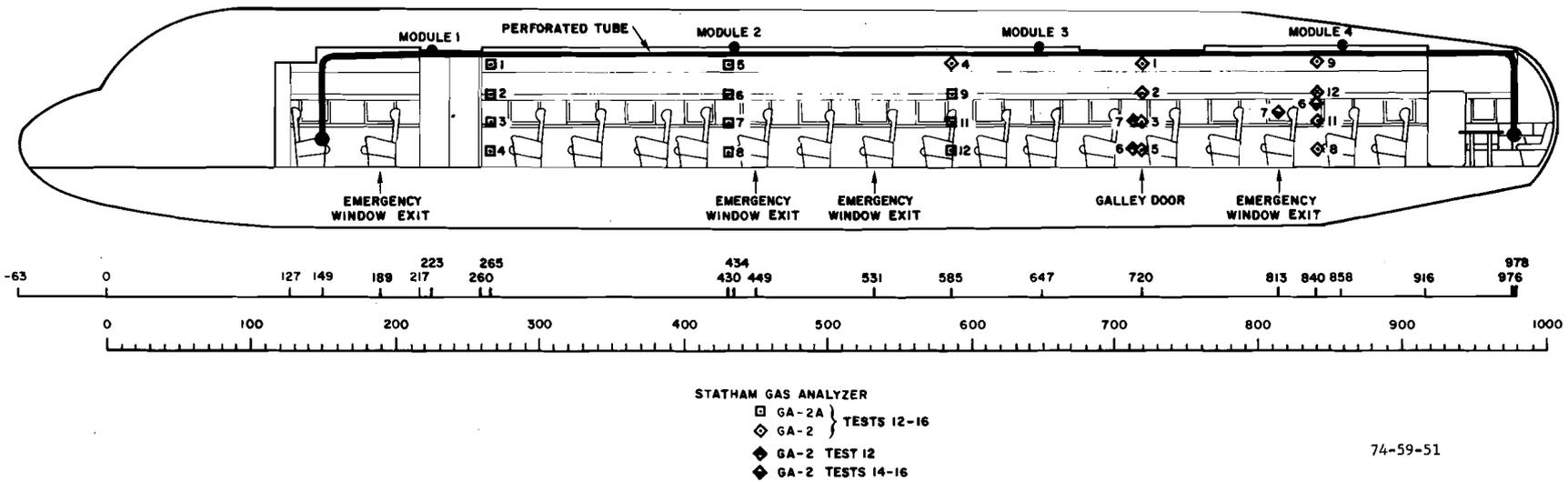
FIGURE 51. SIDE VIEW OF CABIN SHOWING MEASUREMENT LOCATIONS FOR TESTS 12 TO 16
