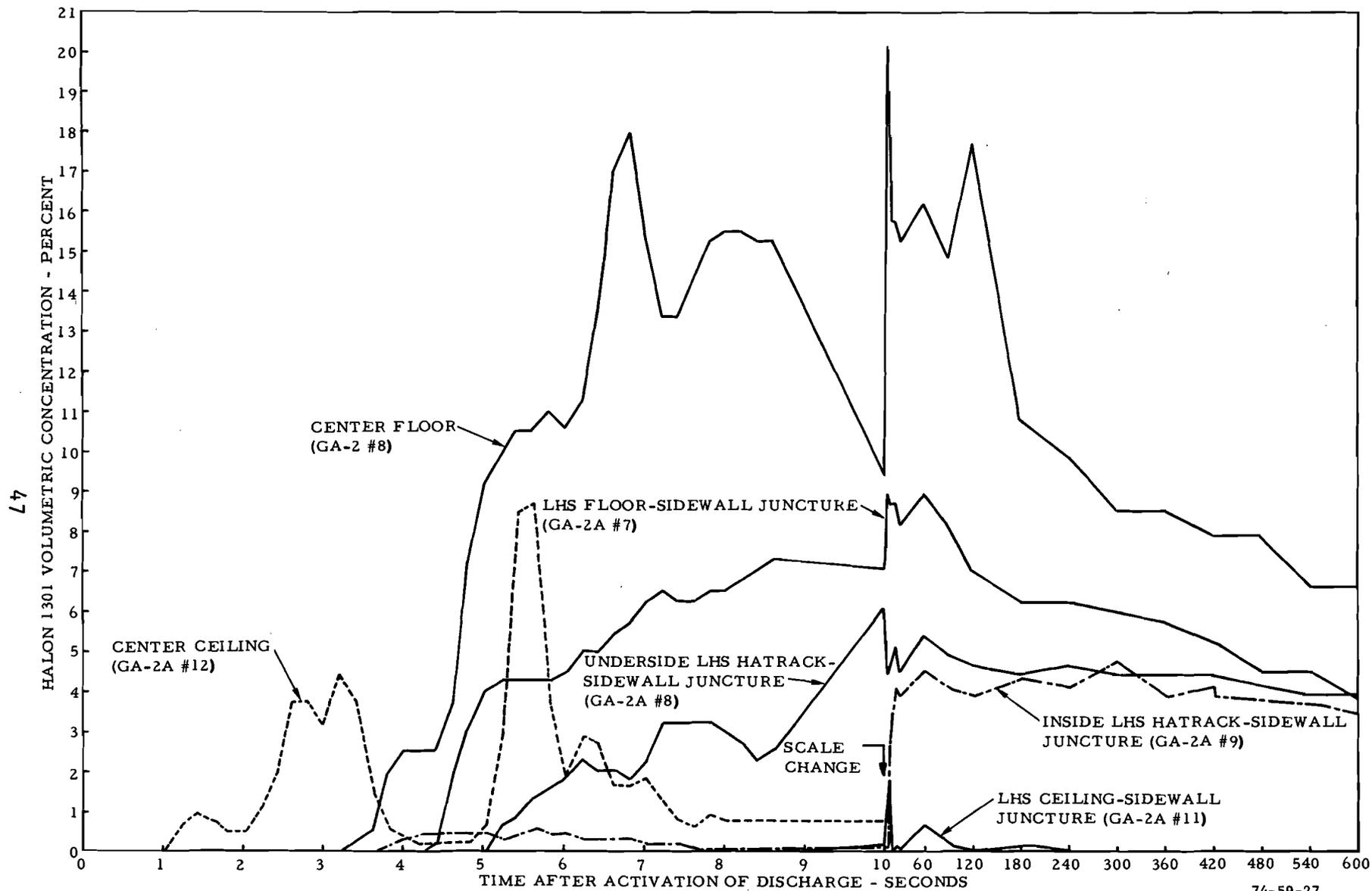
FIGURE 27. HALON 1301 CONCENTRATION AT PERIPHERAL CABIN LOCATIONS AT FUSELAGE STATION 432 FOR THE FOAM-COVERED PERFORATED TUBE SUPPRESSION SYSTEM (TEST 6)
