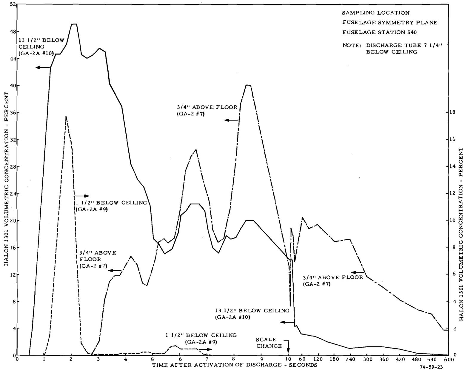
FIGURE 23. HALON 1301 CONCENTRATION ABOVE (GA-2A #9) AND BELOW (GA-2A #10, GA-2 #7) THE FOAM-COVERED PERFORATED DISCHARGE TUBE AT FUSELAGE STATION 540 DURING TEST 5
