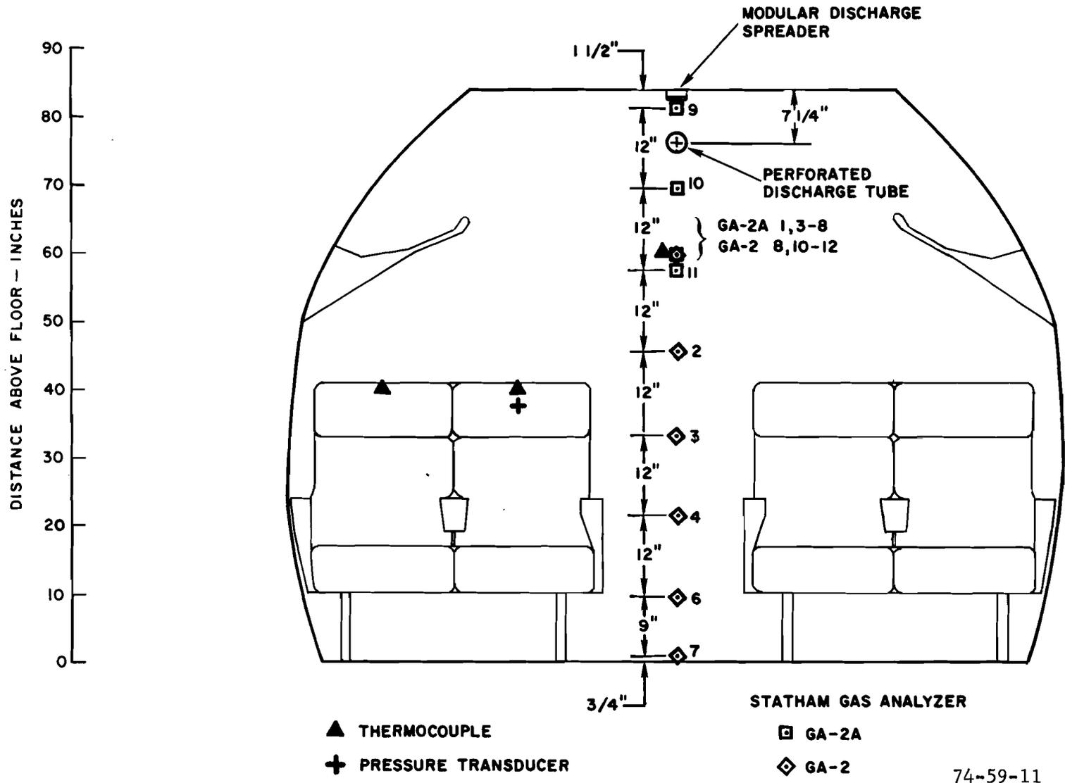
FIGURE 11. CROSS SECTIONAL VIEW OF CABIN SHOWING MEASUREMENT LOCATIONS FOR TESTS 2 TO 5
