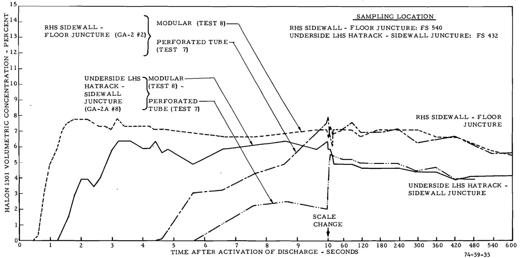
FIGURE 35. HALON 1301 BUILDUP AT CABIN LOCATIONS SHIELDED FROM THE DIRECT DISCHARGE OF THE MODULAR AND PERFORATED SUPPRESSION SYSTEMS
