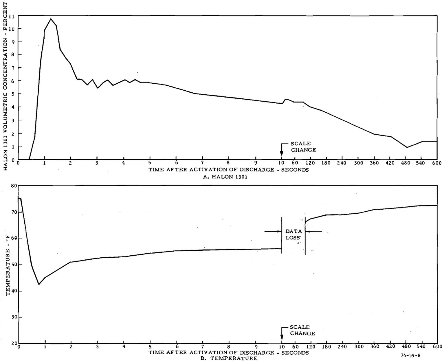
FIGURE 8. HALON 1301 CONCENTRATION AND TEMPERATURE IN THE FUSELAGE SYMMETRY PLANE AT FUSELAGE STATION 545 AT A DISTANCE OF 5 FEET ABOVE THE FLOOR FOR THE MODULAR SUPPRESSION SYSTEM (TEST 1)
