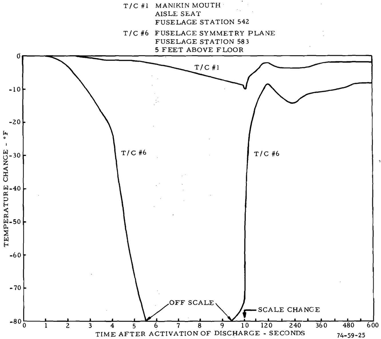
FIGURE 25. CABIN TEMPERATURE CHANGE ASSOCIATED WITH DISCHARGE FROM THE FOAM-COVERED PERFORATED TUBE SYSTEM (TEST 5)
