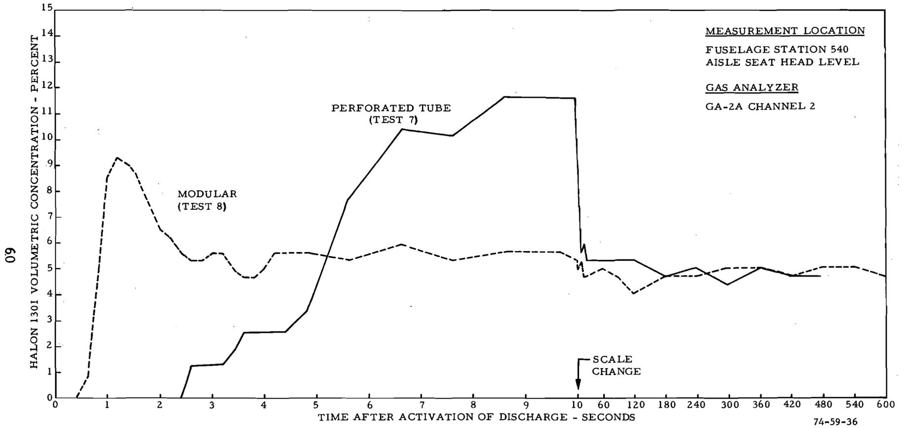
FIGURE 36. HALON 1301 EXPOSURE LEVEL FOR A SEATED PASSENGER COMPARED FOR MODULAR AND PERFORATED TUBE DISPERSERS
