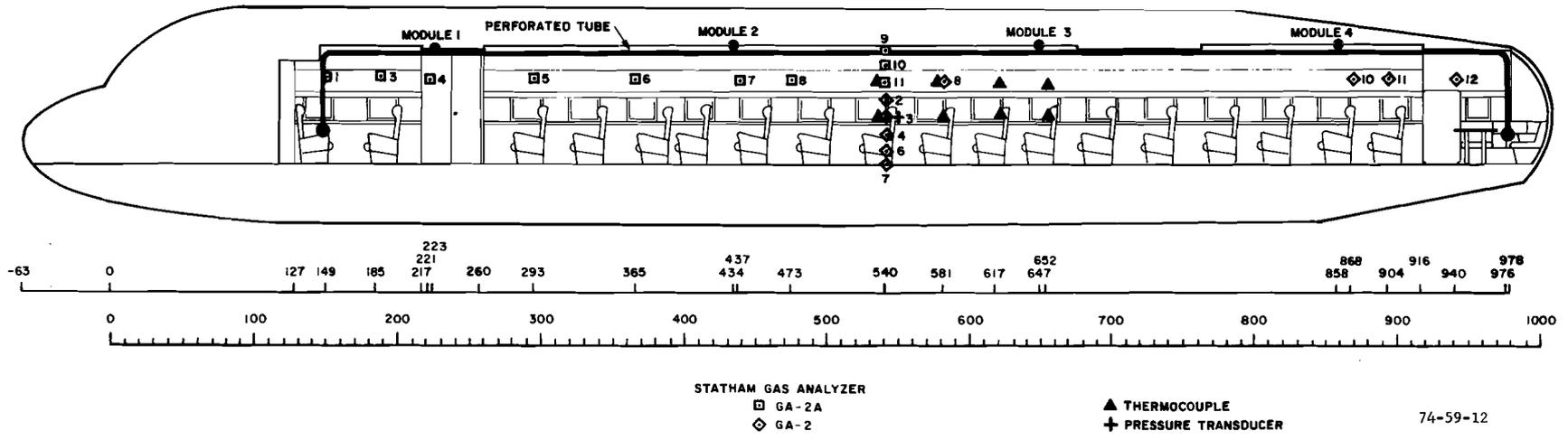
FIGURE 12. SIDE VIEW OF CABIN SHOWING MEASUREMENT LOCATIONS FOR TESTS 2 TO 5
