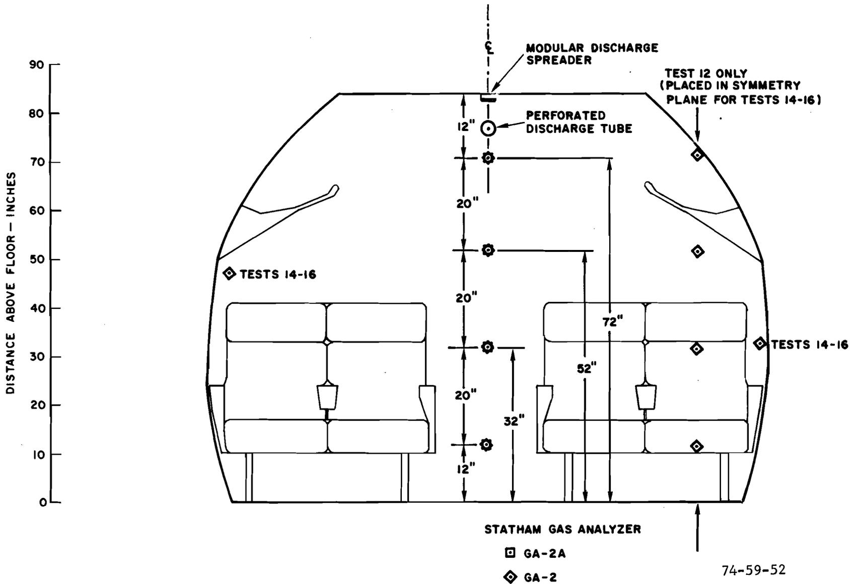
FIGURE 52. CROSS SECTIONAL VIEW OF CABIN SHOWING MEASUREMENT LOCATIONS FOR TESTS 12 TO 16
