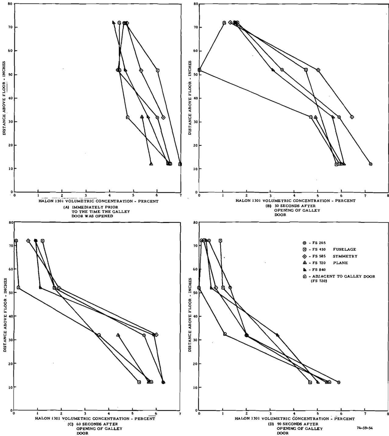
FIGURE 54. VERTICAL HALON 1301 PROFILES AT VARIOUS FUSELAGE STATIONS FOR TEST 12
