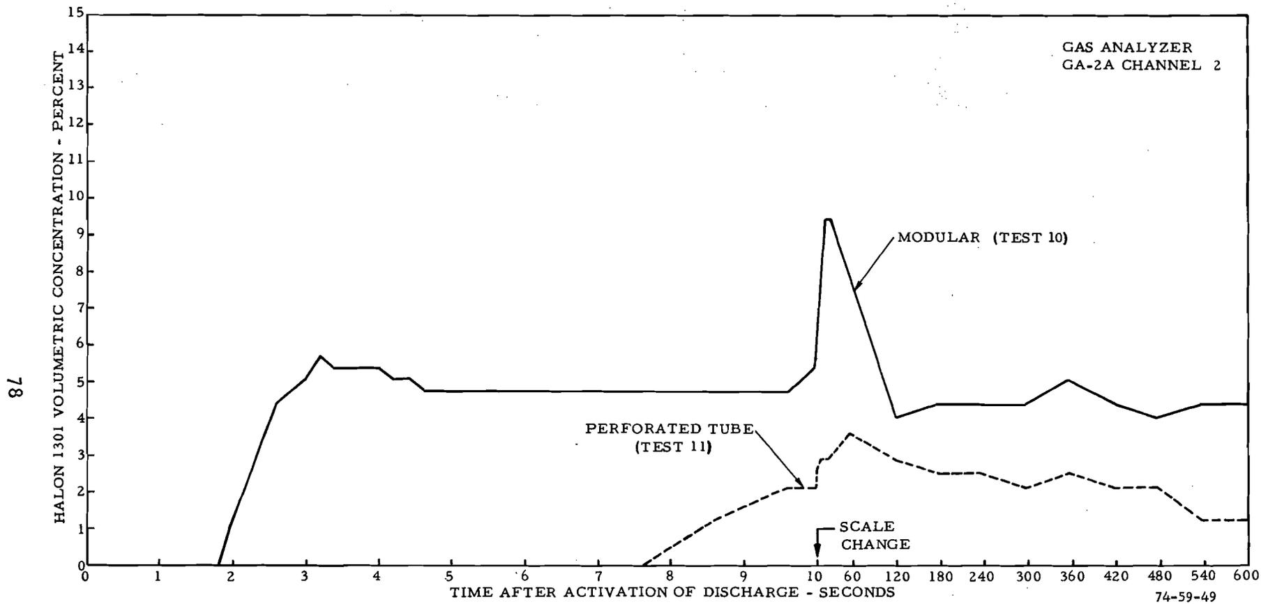
FIGURE 49. COMPARISON OF HALON 1301 BUILDUP IN THE TOWEL DISPENSER OF THE OPEN LAVATORY FOR THE MODULAR AND PERFORATED TUBE SUPPRESSION SYSTEMS
