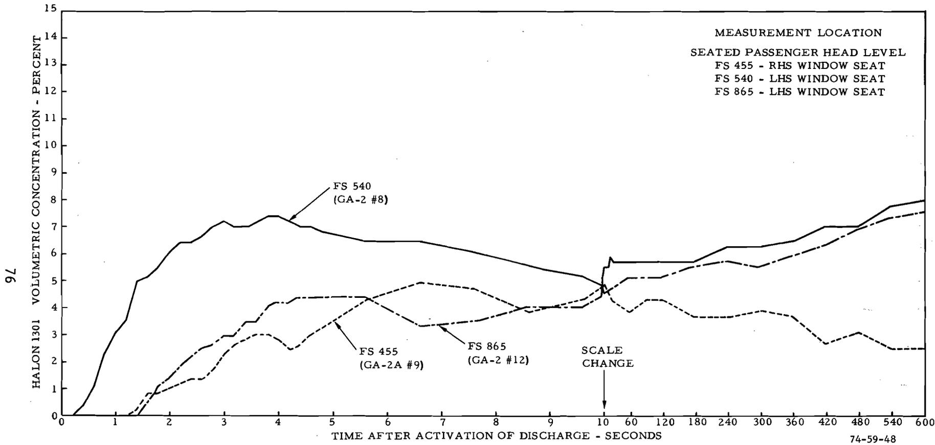
FIGURE 48. HALON 1301 CONCENTRATION-TIME PROFILES NEAR SEATED PASSENGERS DURING TEST 10 (MODULAR SUPPRESSION SYSTEM)
