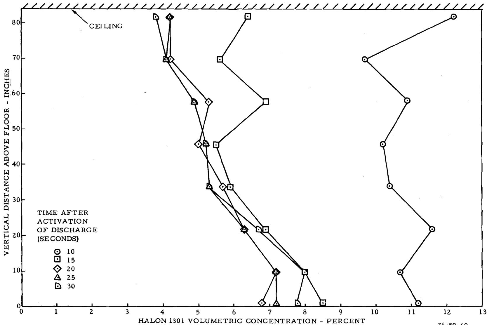
FIGURE 40. VERTICAL HALON 1301 PROFILES AT FUSELAGE STATION 540 SHORTLY AFTER ACTIVATION OF DISCHARGE FROM THE PERFORATED TUBE SUPPRESSION SYSTEM (TEST 9)
