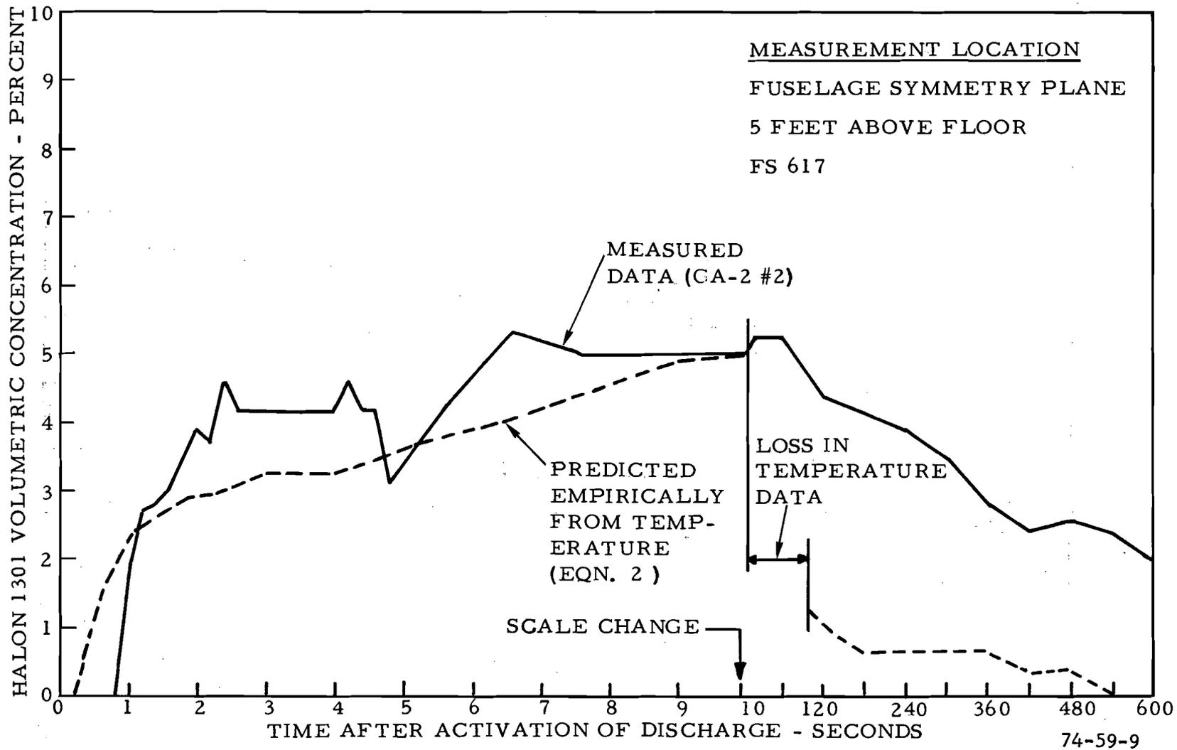
FIGURE 9. A COMPARISON OF HALON 1301 CONCENTRATION MEASURED AND PREDICTED EMPIRICALLY FROM THERMOCOUPLE DATA
