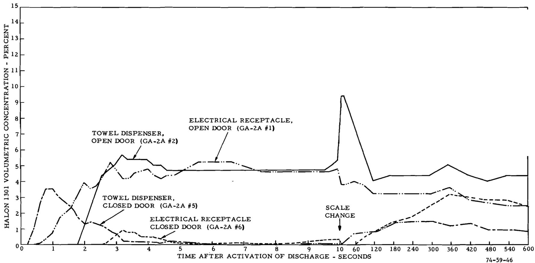
FIGURE 46. COMPARISON OF AGENT BUILDUP IN THE LAVATORY WITH THE DOOR OPEN AND CLOSED FOR THE MODULAR SUPPRESSION SYSTEM (TEST 10)
