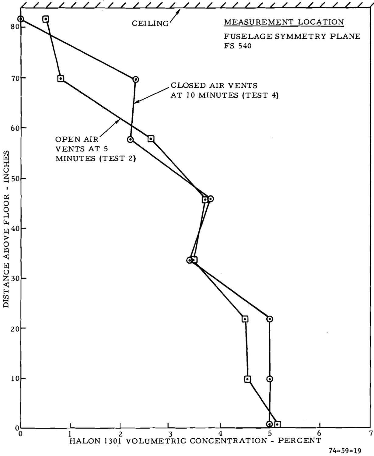
FIGURE 18. AN INDICATION OF THE EXTENSION IN INERTING PROTECTION PROVIDED BY CLOSING THE AIR VENTS
