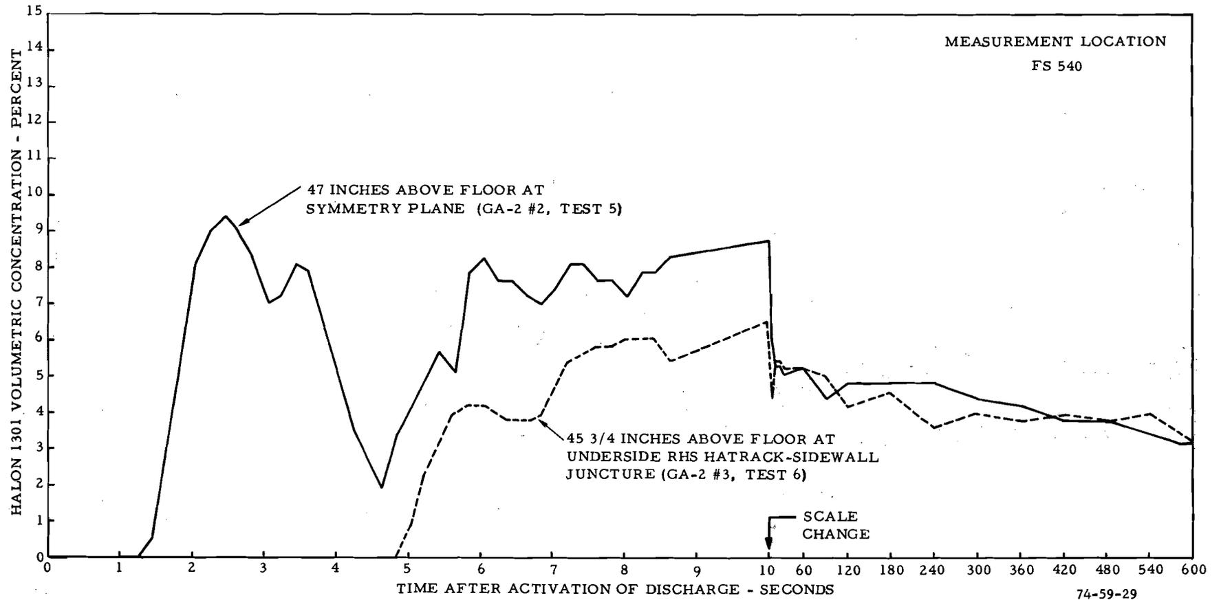
FIGURE 29. COMPARISON OF HALON 1301 CONCENTRATION AT SYMMETRY PLANE AND SIDEWALL LOCATIONS EQUIDISTANT ABOVE THE FLOOR FOR THE FOAM-COVERED PERFORATED TUBE SUPPRESSION SYSTEM
