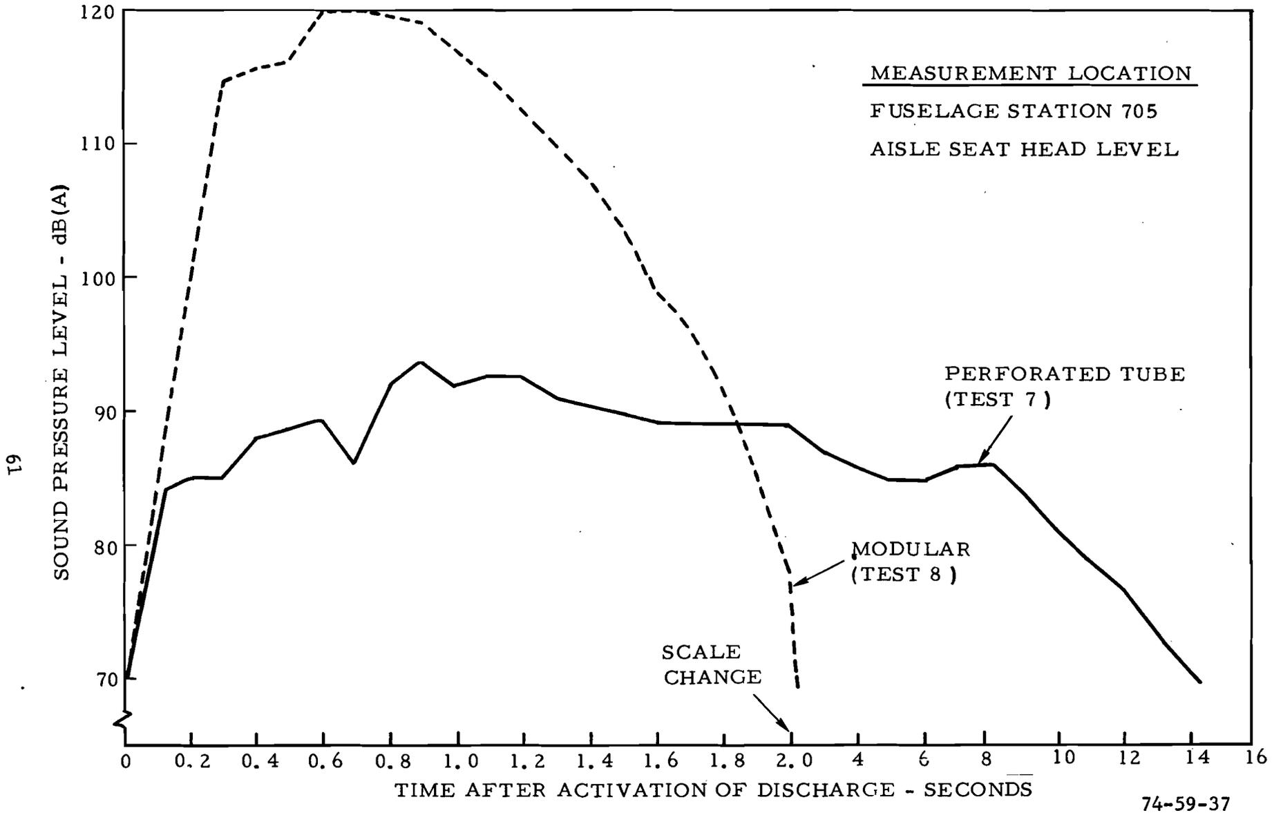
FIGURE 37. CABIN NOISE DURING HALON 1301 DISCHARGE FROM MODULAR AND PERFORATED TUBE DISPERSERS
