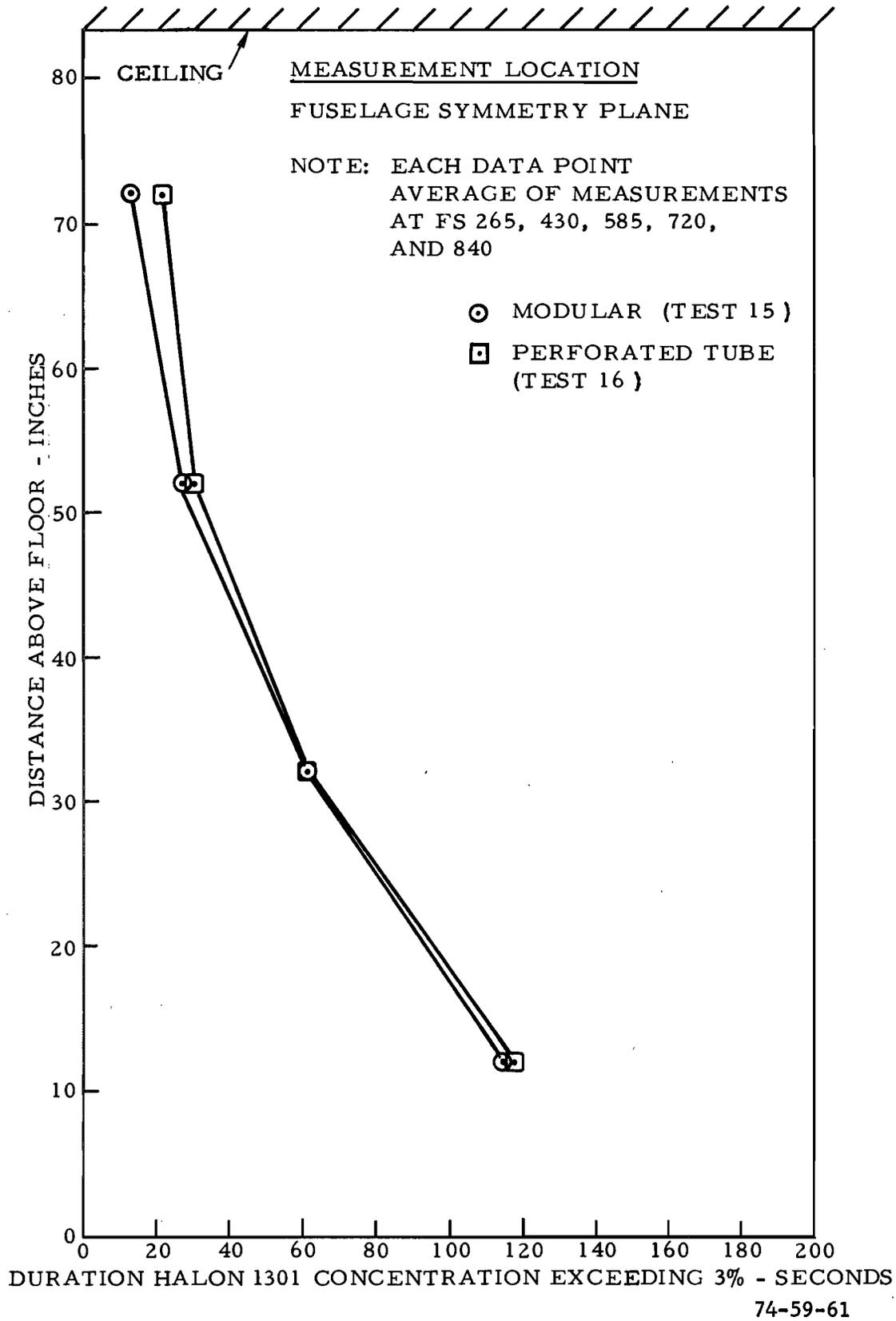
FIGURE 61. COMPARISON OF AVERAGE VERTICAL HALON 1301 PROFILES FOR THE MODULAR (TEST 15) AND PERFORATED TUBE (TEST 16) SYSTEMS WHEN ALL LHS EXITS ARE OPEN AT TIME OF DISCHARGE ACTIVATION
