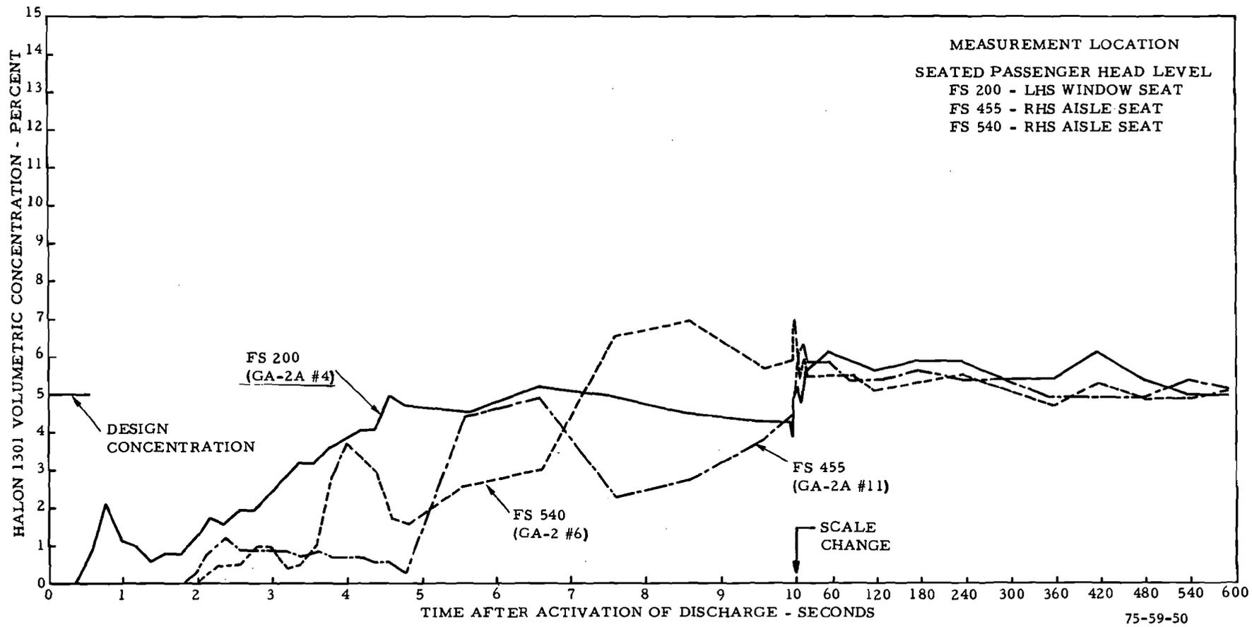
FIGURE 50. HALON 1301 CONCENTRATION-TIME PROFILES NEAR SEATED PASSENGERS DURING TEST 11 (PERFORATED TUBE SUPPRESSION SYSTEM)
