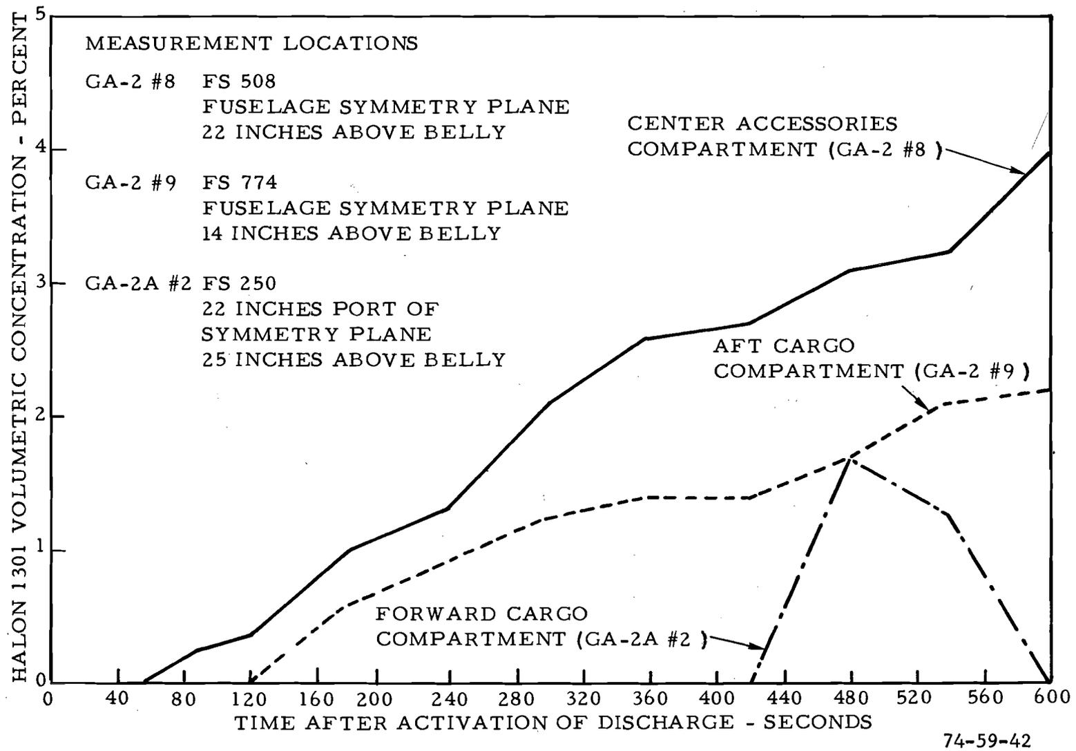
FIGURE 42. AGENT LEAKAGE INTO COMPARTMENTS BELOW MAIN CABIN FLOOR (TEST 9)
