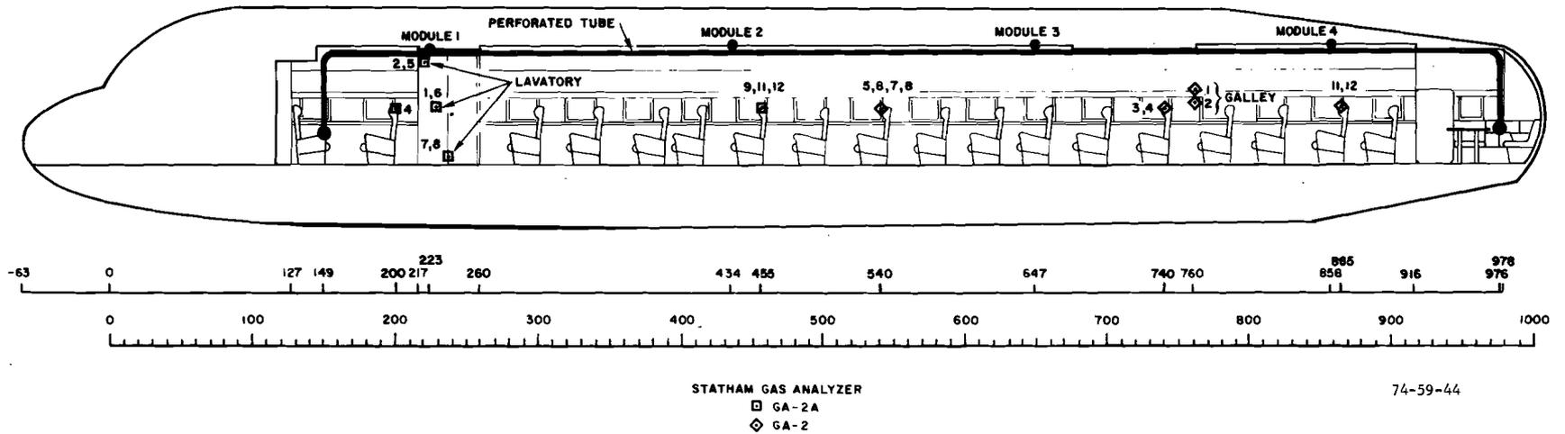
FIGURE 44. SIDE VIEW OF CABIN SHOWING MEASUREMENT LOCATIONS FOR TESTS 10 AND 11
