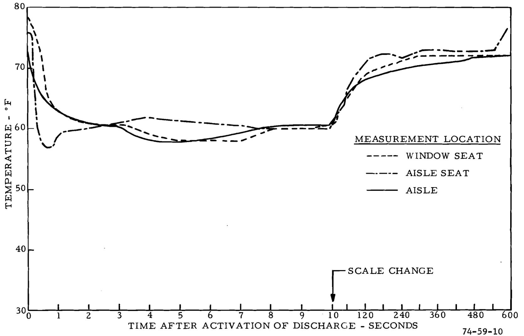
FIGURE 10. SIMILARITY IN THE CABIN TEMPERATURE MEASURED AT THE HEAD LEVEL OF PASSENGERS AT FUSELAGE STATION 652 (TEST 1)
