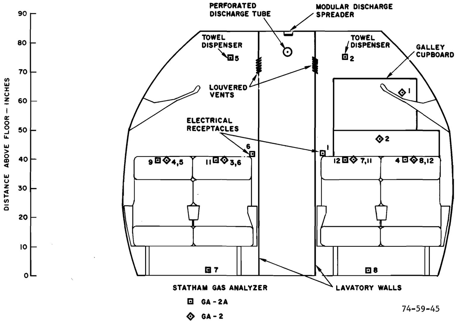
FIGURE 45. CROSS SECTIONAL VIEW OF CABIN SHOWING MEASUREMENT LOCATIONS FOR TESTS 10 AND 11
