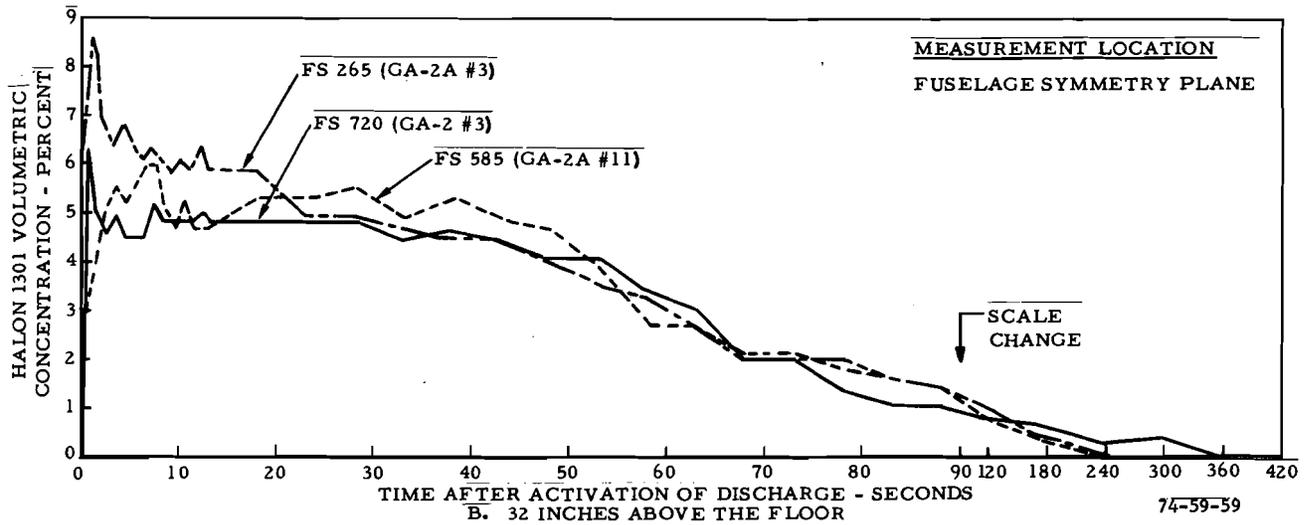
FIGURE 59. COMPARISON OF HALON 1301 CONCENTRATION-TIME PROFILES AT VARIOUS FUSELAGE STATIONS WHEN THE LHS EXITS ARE OPEN AT DISCHARGE ACTIVATION FROM THE MODULAR SYSTEM (TEST 15)
