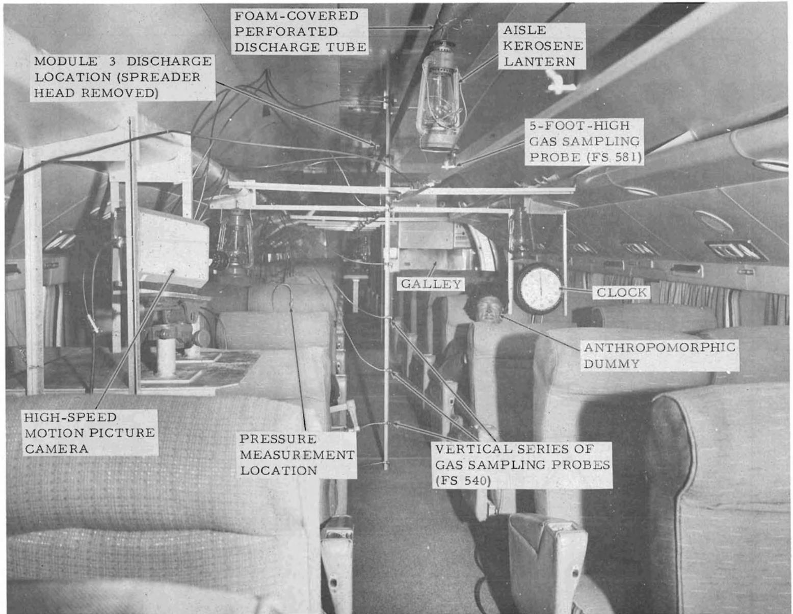
FIGURE 17. PHOTOGRAPH OF CABIN INTERIOR LOOKING AFT FROM FS 365 BEFORE TEST 4
