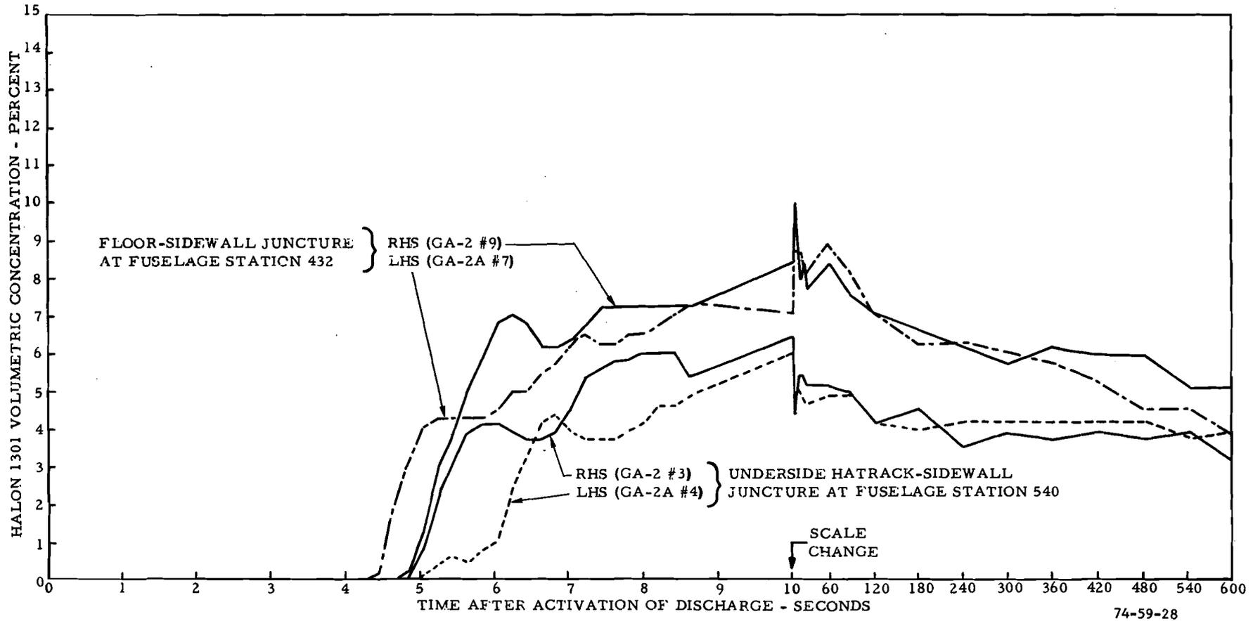
FIGURE 28. LATERAL SYMMETRY OF HALON 1301 CONCENTRATION DISTRIBUTION AT PERIPHERAL CABIN LOCATIONS FOR THE FOAM-COVERED PERFORATED TUBE SUPPRESSION SYSTEM (TEST 6)
