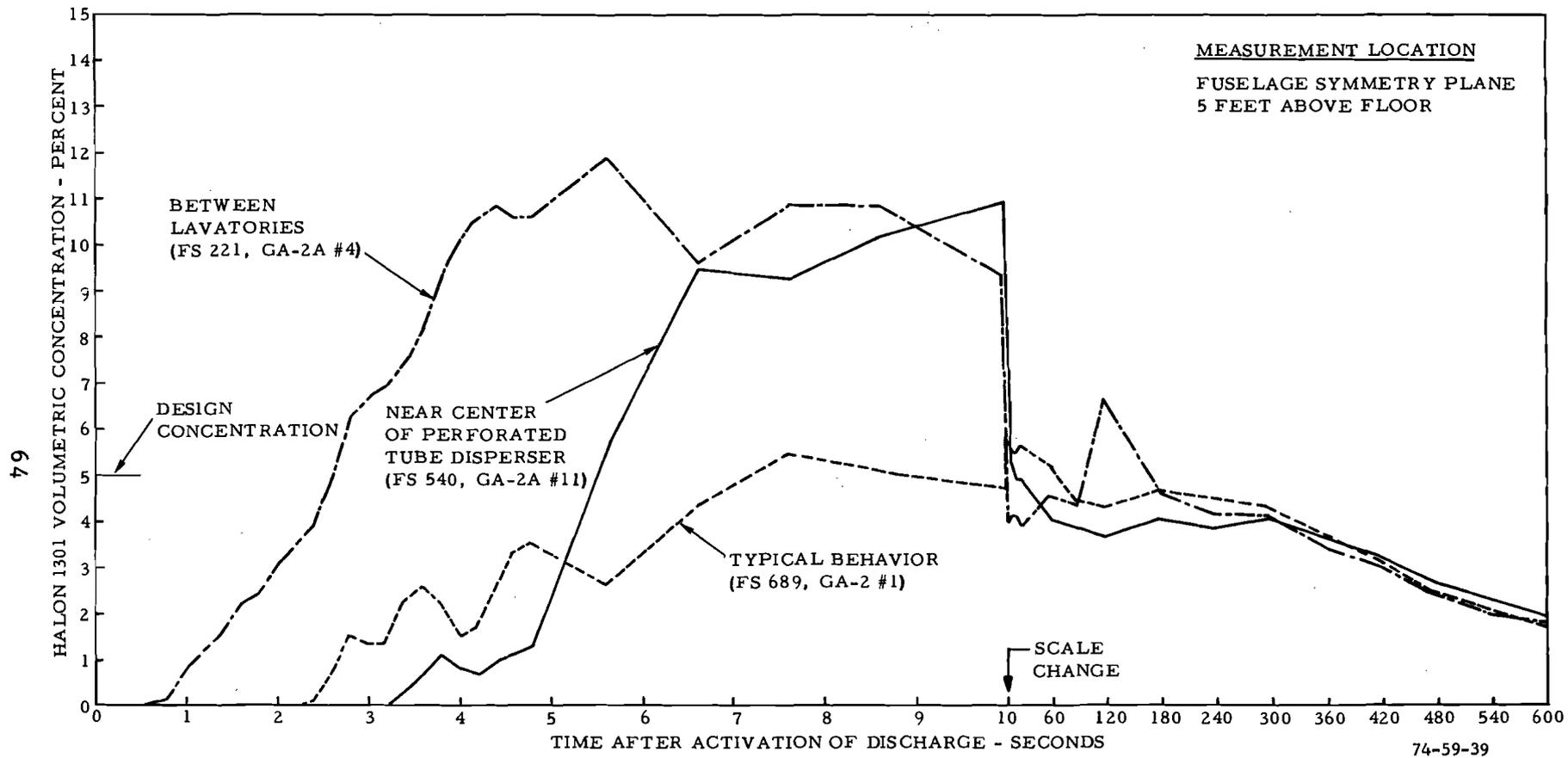
FIGURE 39. HALON 1301 CONCENTRATION-TIME PROFILES AT VARIOUS CABIN LOCATIONS FOR THE PERFORATED TUBE SUPPRESSION SYSTEM (TEST 9)
