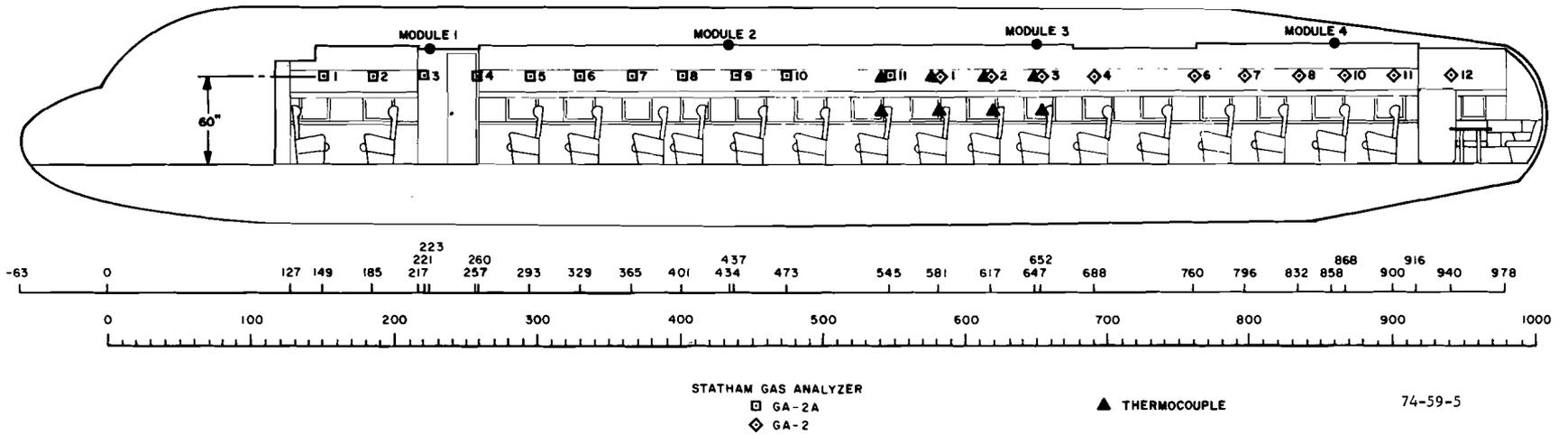
FIGURE 5. LOCATION OF HALON 1301 SAMPLING LINES IN THE FUSELAGE SYMMETRY PLANE AND THERMOCOUPLES FOR TEST 1
