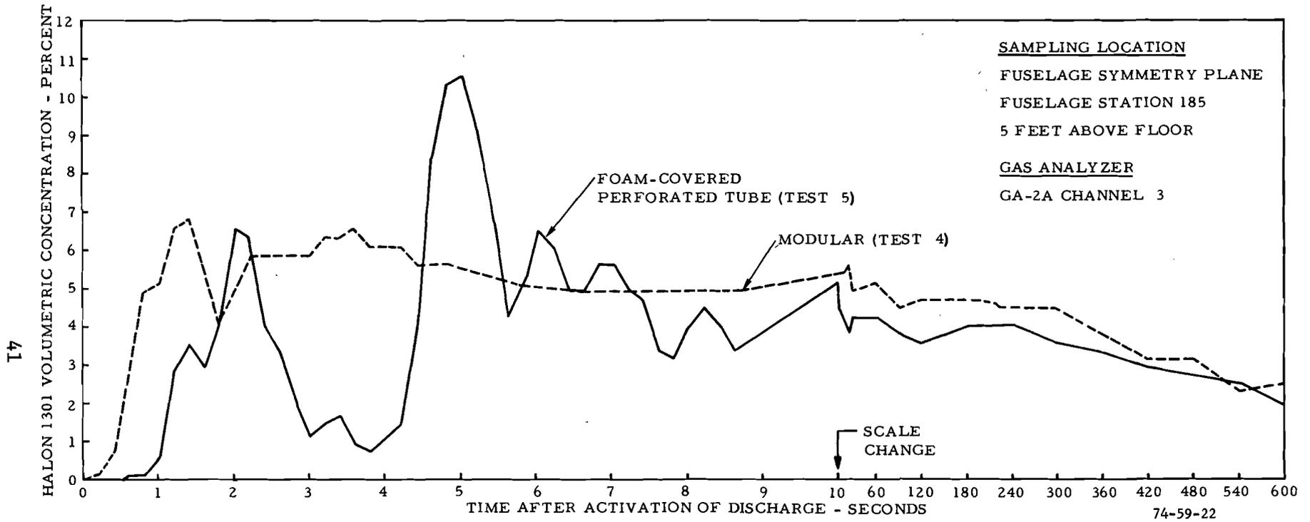
FIGURE 22. HALON 1301 CONCENTRATION IN "B" LOUNGE COMPARED FOR MODULAR (TEST 4) AND FOAM-COVERED PERFORATED TUBE (TEST 5) SUPPRESSION SYSTEMS
