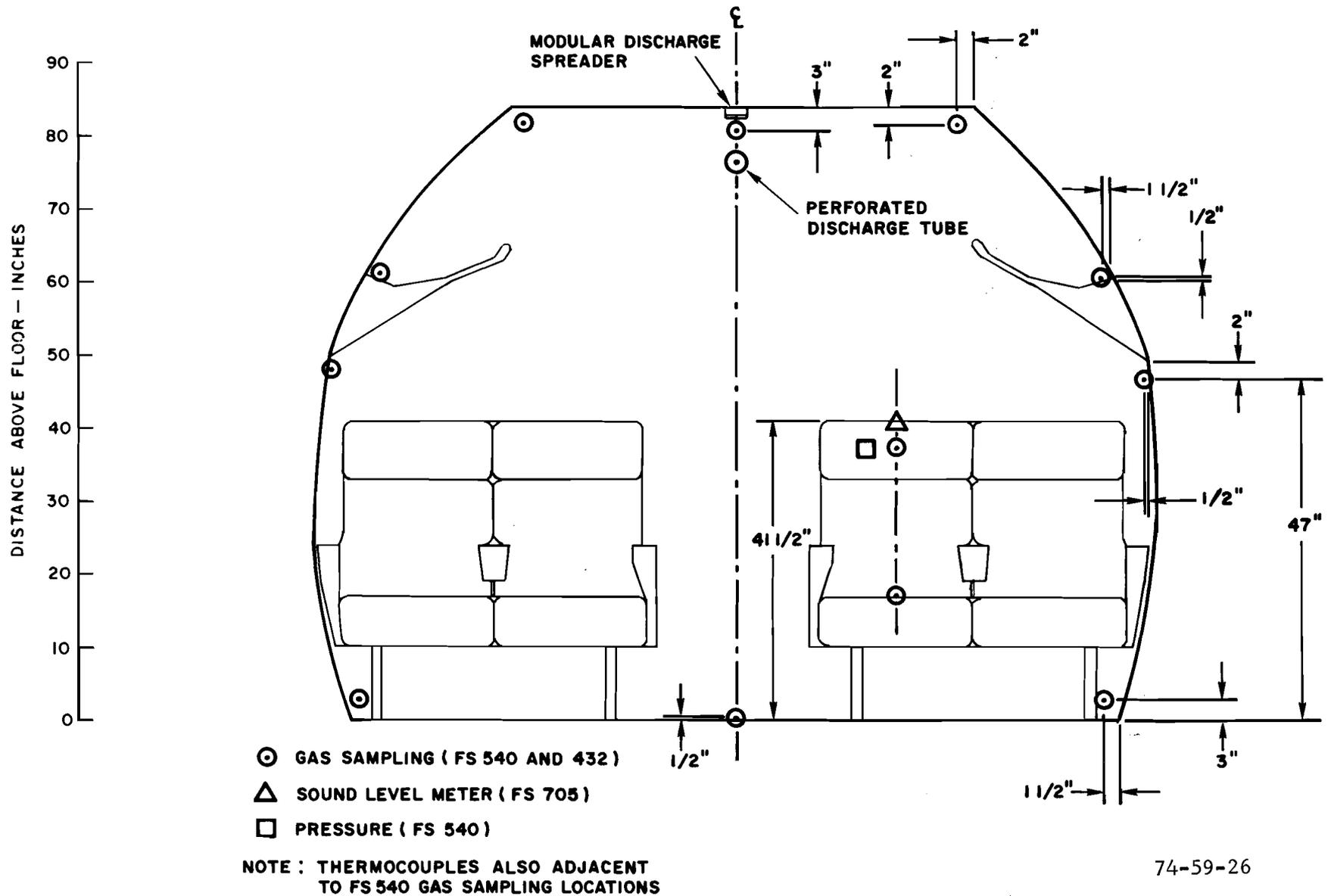
FIGURE 26. CROSS SECTIONAL VIEW OF CABIN SHOWING MEASUREMENT LOCATIONS FOR TESTS 6 TO 8
