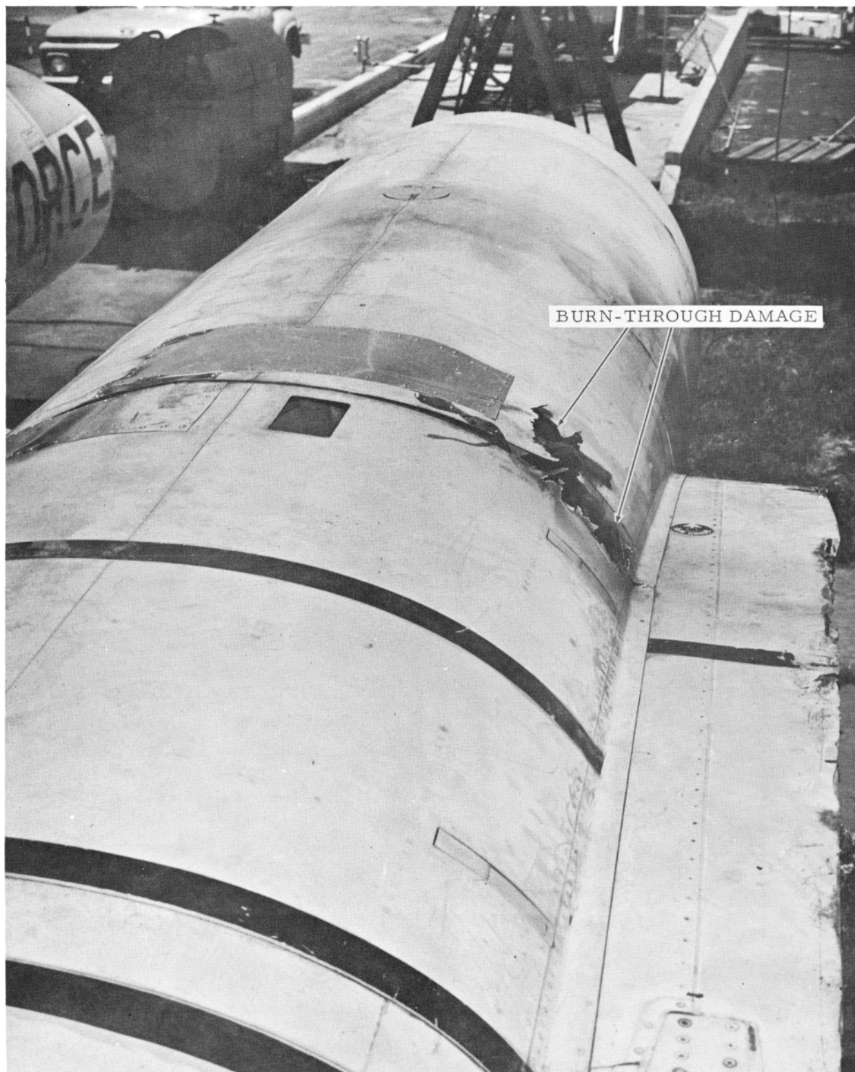
FIGURE 26. DAMAGE TO COWLING FROM BURN-THROUGH (TEST NO. 3)
