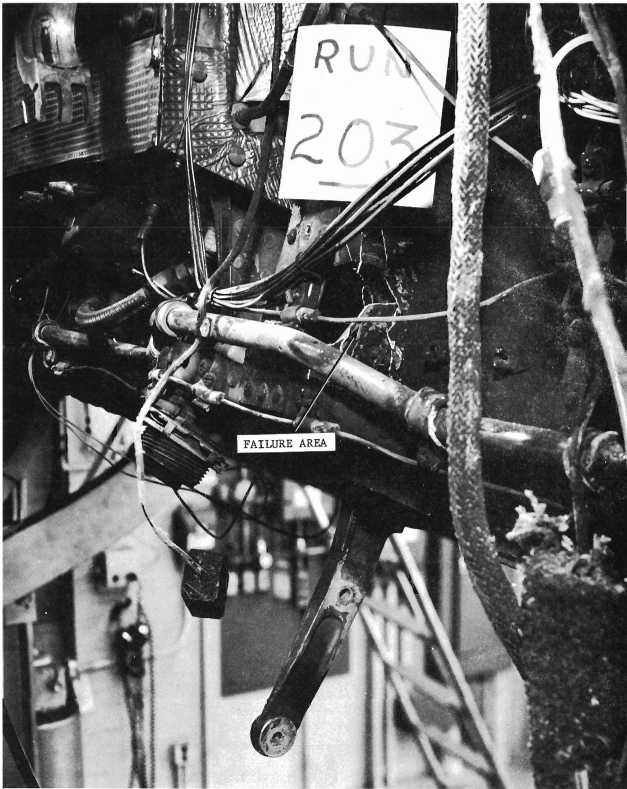
FIG. 20 DAMAGE TO ZONE II MAIN ACCESS DOOR AFT HINGE SUPPORT BRACKET
