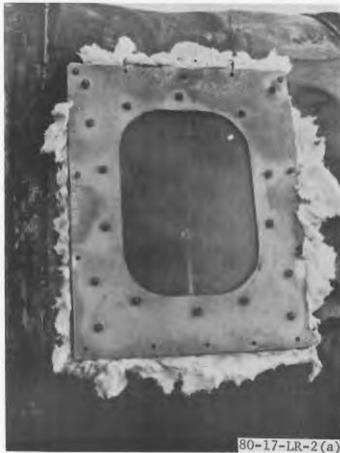
WINDOW SEGMENTS WITH CALORIMETERS (TESTS 3 AND 4)
