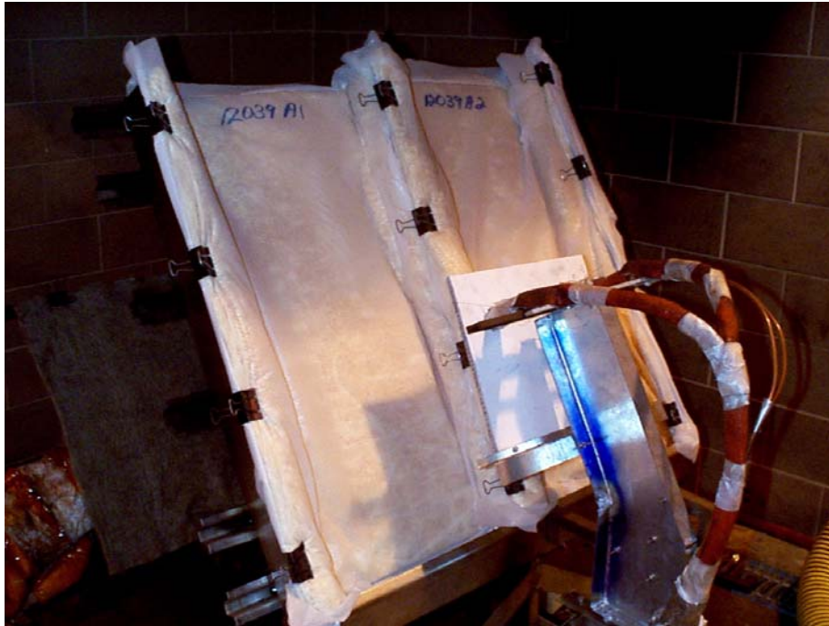
Figure 13. Position of 12 Spring Clamps Used to Mount Insulation Blanket Samples
