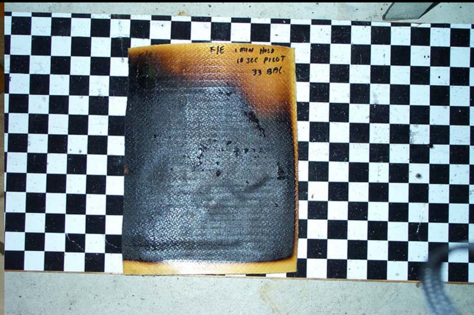
WJH FAA Tech Center Test 012705T02 Kevlar/Epoxy
