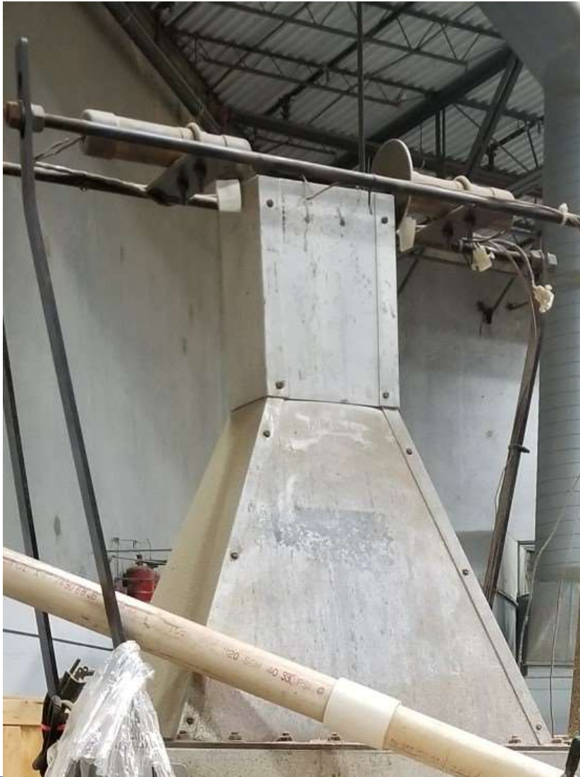
Heat Release Rate Test Apparatus October 2023
