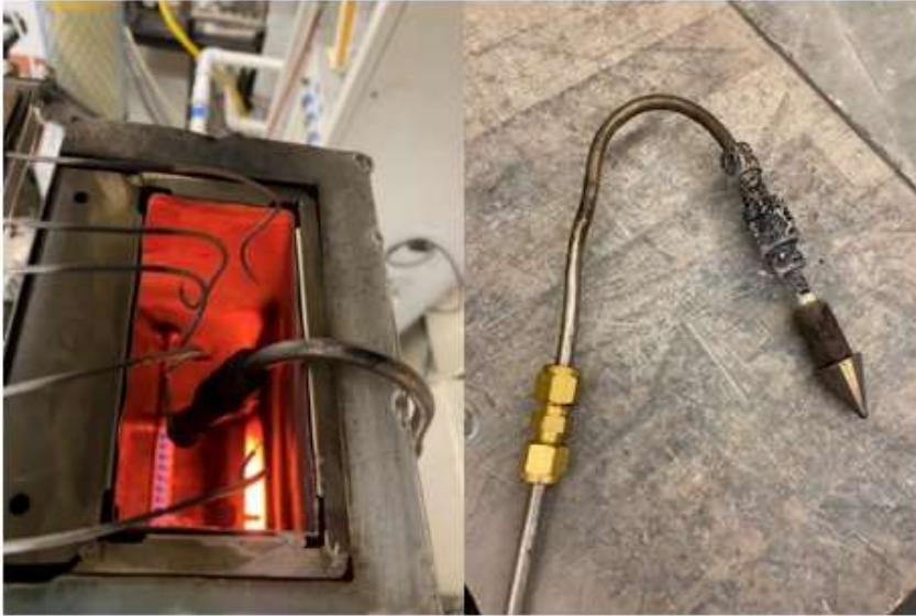
Hydrogen Sample Probe Inserted in Exhaust Stream
