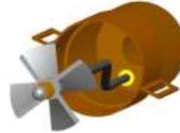
Figure 7-5-15. Location of the Stator on the Fuel Tube
