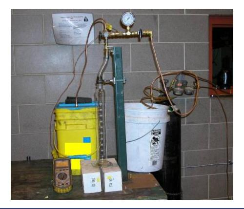
Fuel is pressurized to 100 psi, and fuel is collected for one minute then stopped. The reading on the graduated cylinder shows the number of milliliters that flow in one minute. This is then converted to gallons per hour. The actual fuel flow rate can then be compared to the rated flow rate of the nozzle. A higher quality nozzle will show a lower difference between actual and rated flow rates.
