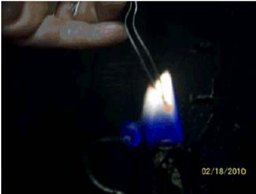
Thermocouple Measurement taken from center of flame.
