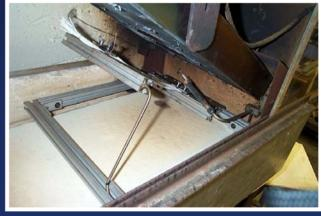
The center of the pilot burner flame must impinge the wire at a distance of no more than 5 inches (12.7 cm) from the lower clamping point.
