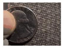
FILLING: compound required to fill the voids created by the fabric weave.
