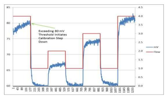
(Graphs are for demonstration purposes only) <u>"Ramp" Method: This is the new exploritory calibration method</u>
