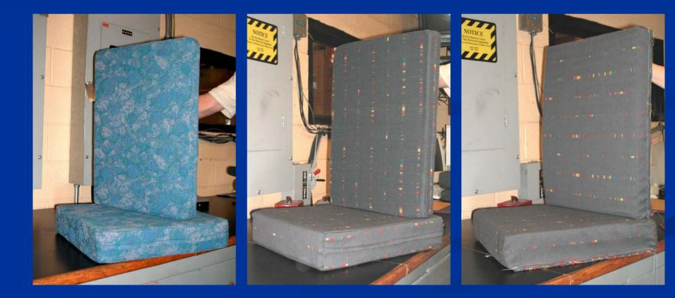
**Aircraft Seats** World Wide Round Robin Testing Testing is complete in the US Testing has started outside the US and we anticipate it will be completed by early May 2007. Data being presented is the Average Percent Weight Loss and it's Standard
