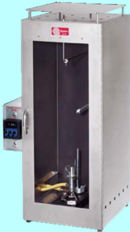
Bunsen Burner Tests
