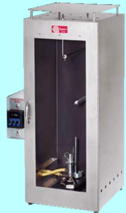
Vertical Flame Test
