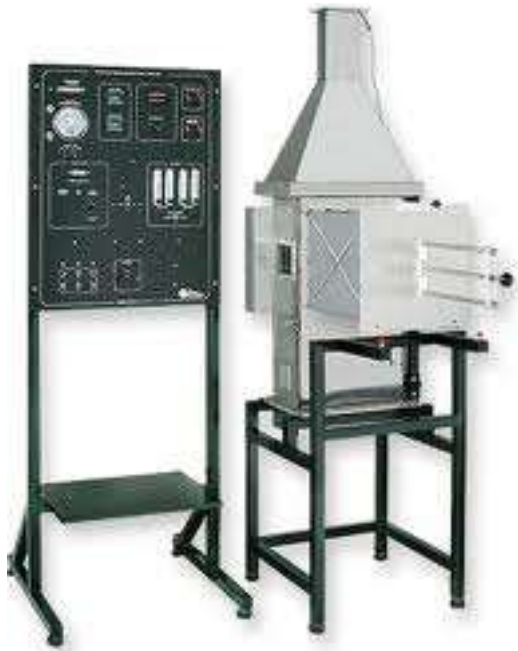
OSU Rate of Heat Release Apparatus (Large Area Materials)
