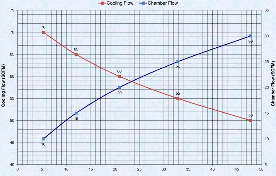
HR2 Plenum Pressure / Cooling Flow / Chamber Flow Correlation (Constant Total Flow of 80 SCFM)
