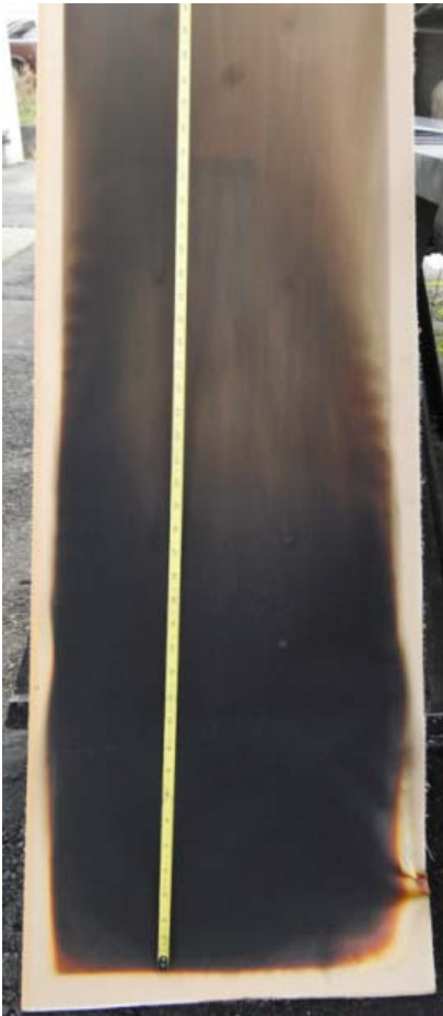
0.25" Honeycomb/ phenolic prepreg
