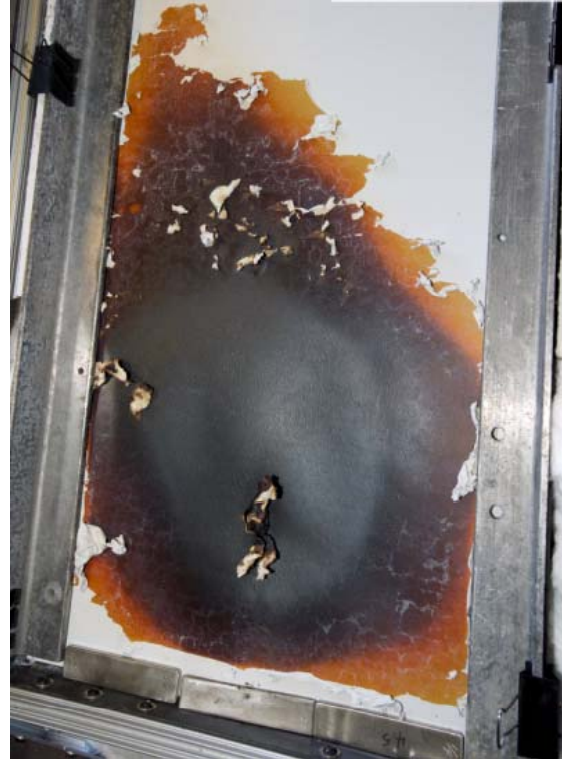
Rigid Cargo Liner (front side). Specimen still in test fixture. Tedlar peeled off during the test.
