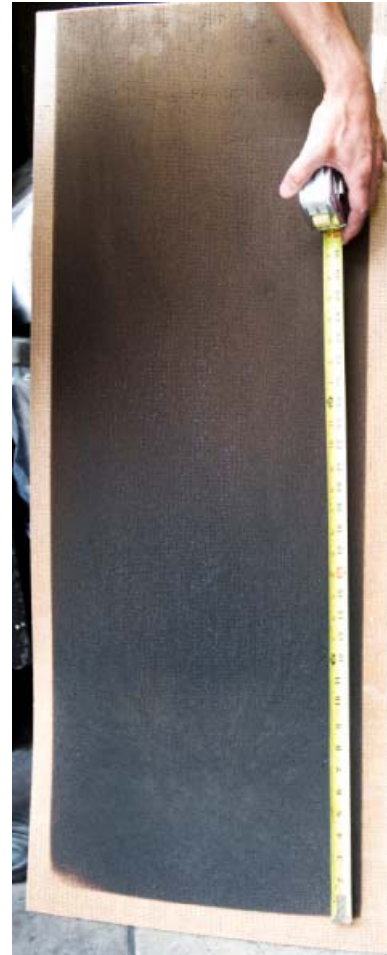
0.10" Side Wall Crushed Core - Test Face
