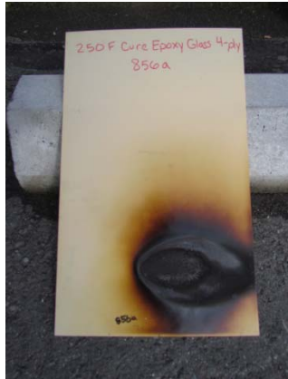
4ply 250F Epoxy Fiberglass
