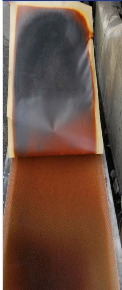
0.25" Honeycomb/ phenolic prepreg
