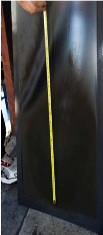
250F cure epoxy carbon fabric 4 ply
