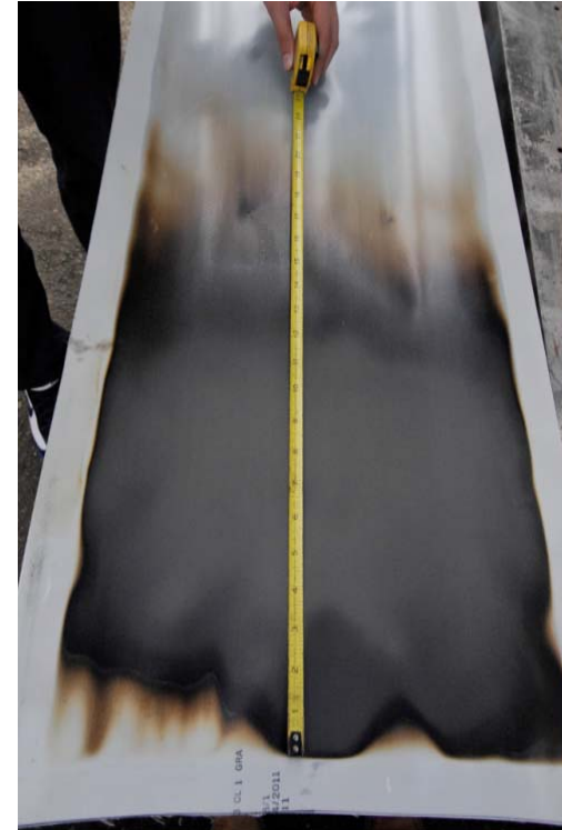
Rigid Cargo Liner, t = 0.013 " - Test side
