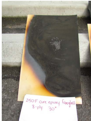
8ply 250F Epoxy Fiberglass
