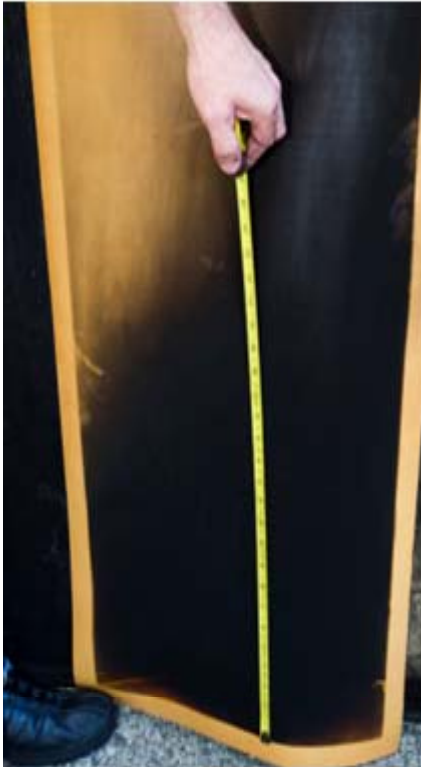
Rigid Cargo Liner, t = 0.013 " - Test side
