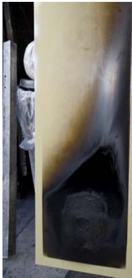
250F Cure Epoxy Fiberglass 14 ply
