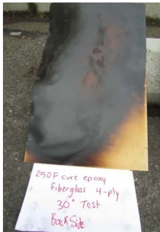
4ply 250F Epoxy Fiberglass
