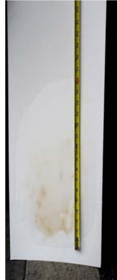
0.10" Side Wall Crushed Core - back
