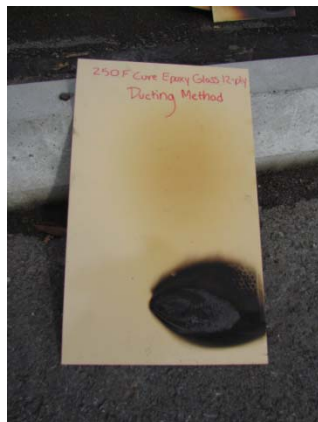
12 ply 250F Epoxy Fiberglass
