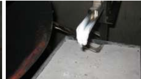
"T" Web Machined from Leg Plate
