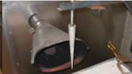
Inverted Cones of AZ-31, Suspended Vertically
