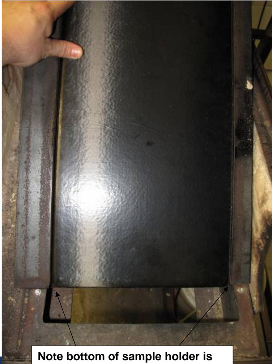
**Note bottom of sample holder is cut out to allow sample to slide down when inclined**
