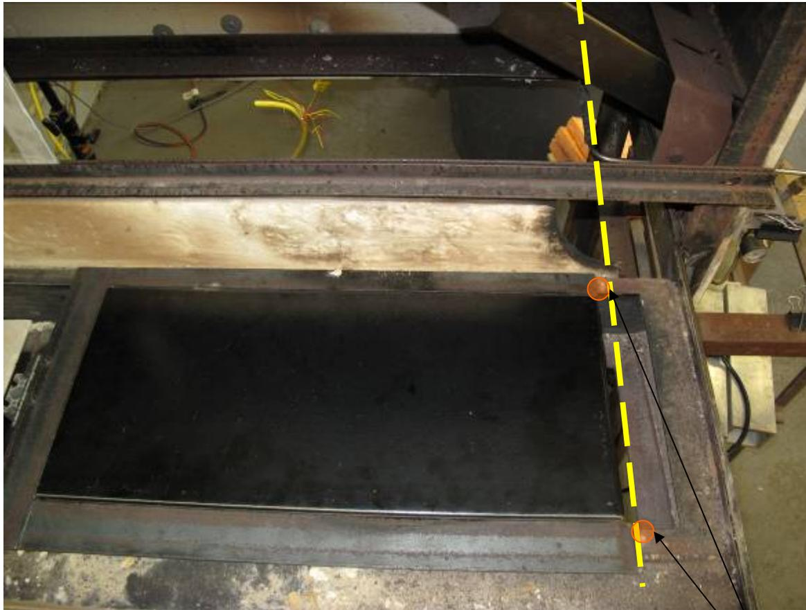
**Two screws are used as stoppers to prevent the sample holder from sliding forward when it tilts up**
