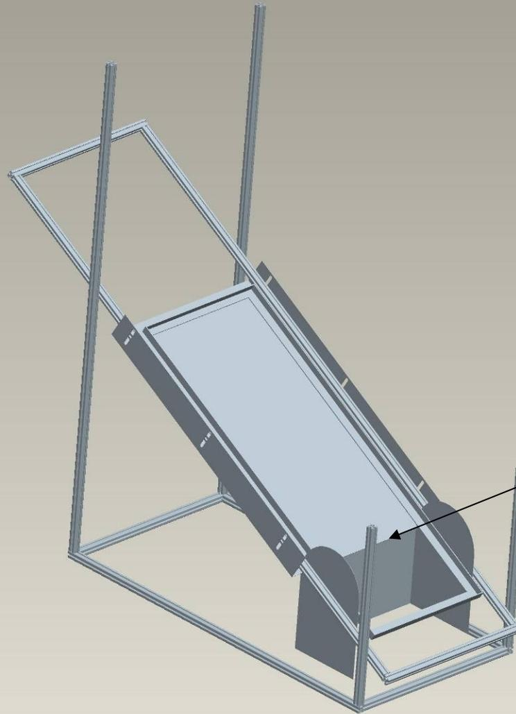
Hinge used to connect shroud with shroud bottom so that shroud bottom is always vertical regardless of angle of panel
