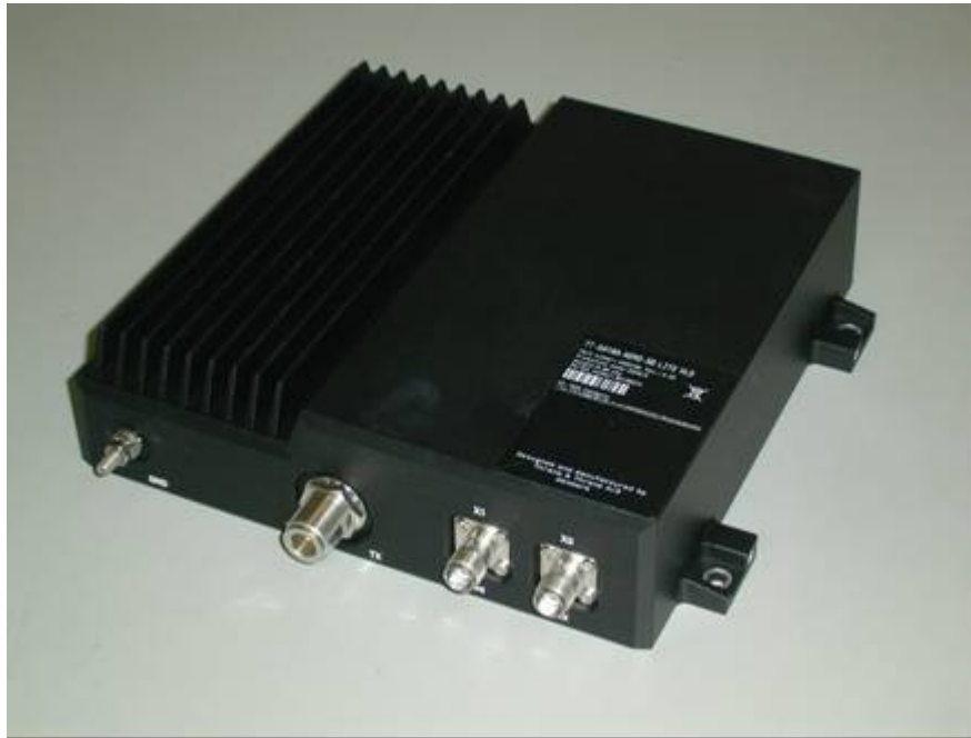
HLD, metal construction with no cooling/vent holes
